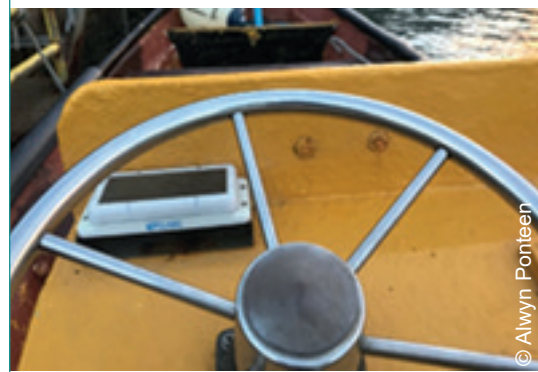
Plate 8. Pelagic IVMS installed on fishing vessel
