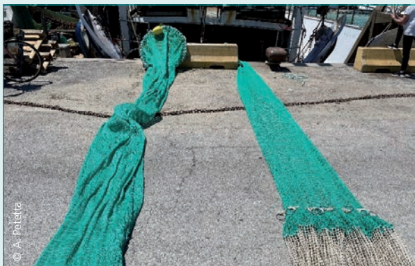
Trawl body made of polyamide.
