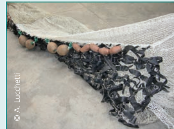
Bottom-side chafer made of black plastic material.
