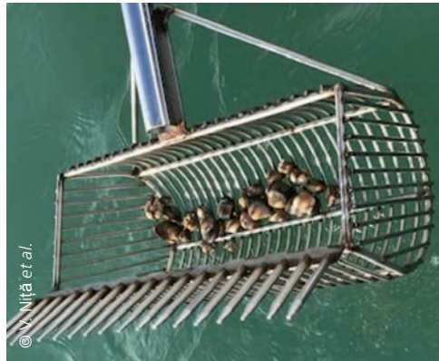
PLATE 48 Hand dredges being tested on the Romanian Black Sea coast to harvest bivalve species
