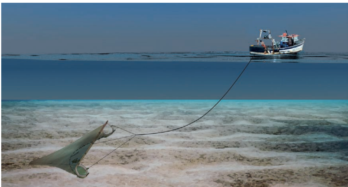
FIGURE 20 Gangui bottom beam trawl used in France
