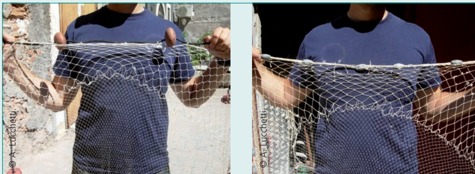
Details of headline and leadline of a menaide used in the southern Tyrrhenian Sea.
