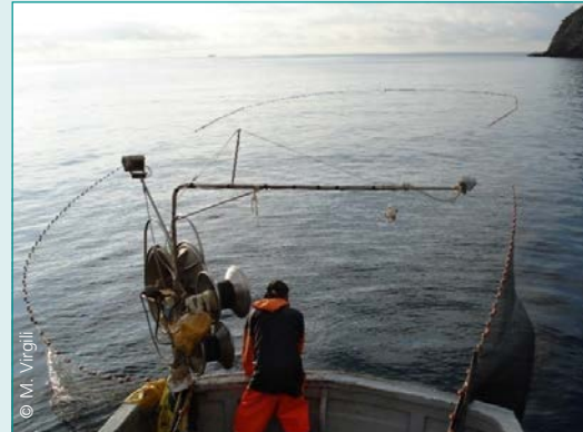
Surrounding net without purse lines during net hauling operations.
