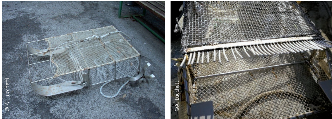
PLATE 35 Viareggino rake mechanized dredge
