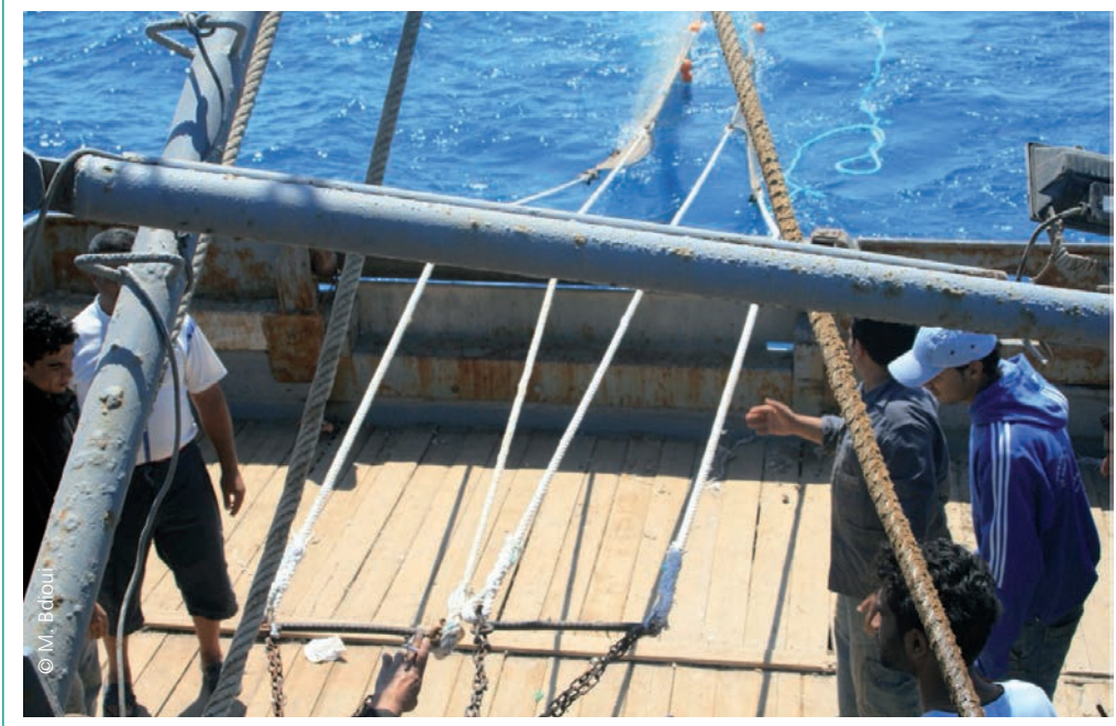
PLATE 6 Trawl net with two bridles used in Tunisia
