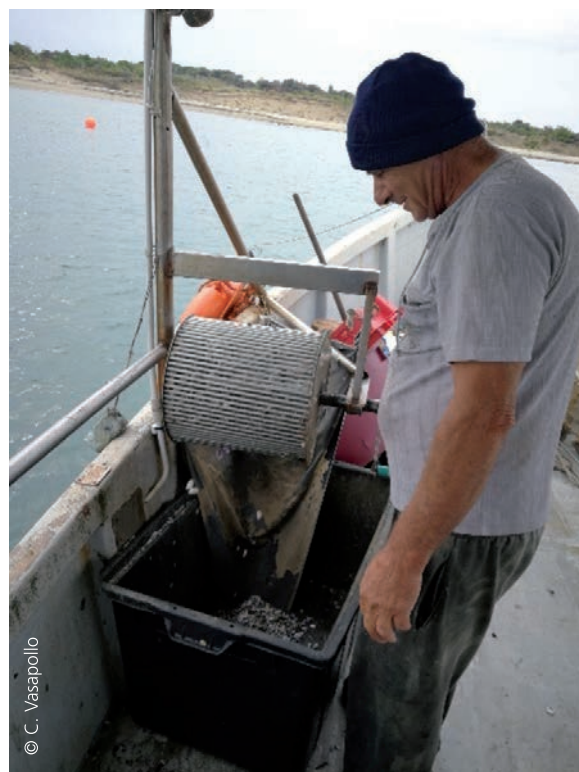
PLATE 36 Manual sieve used on board to sort commercial clams
