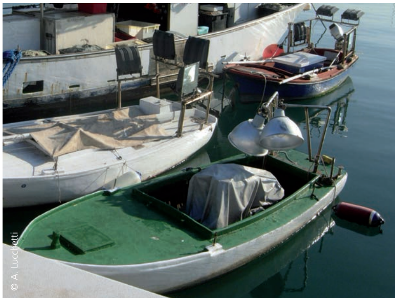
PLATE 18 Tenders equipped with lamps
