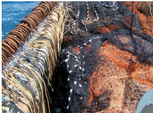
PLATE 17 Purse seine on the stern of a boat with visible purse rings attached to the leadline
