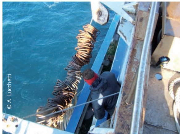
PLATE 20 Recovery of the purse line during hauling
