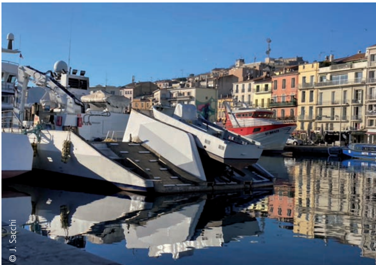
PLATE 26 Skiff on the ramp of a tuna purse seiner used in France
