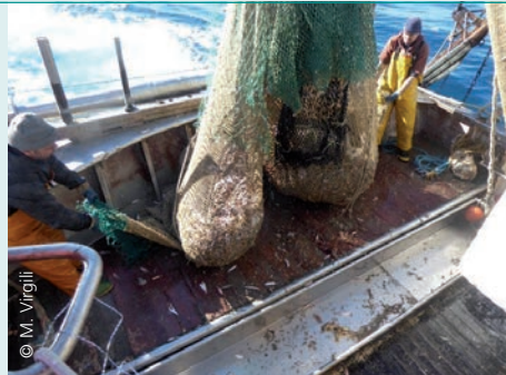
Double codend (or divided codend) used to split catch and provide better-quality catch.
