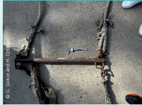
Danleno stick between the headrope and leadrope.
