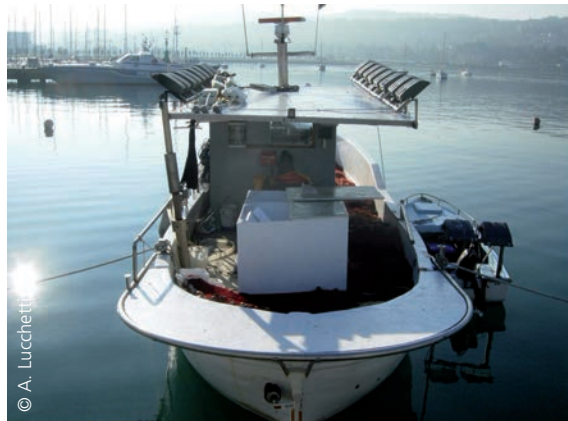
PLATE 19 Purse seiner and adjacent skiff equipped with lamps
