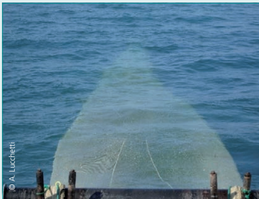
Trawl body made of polyamide.
