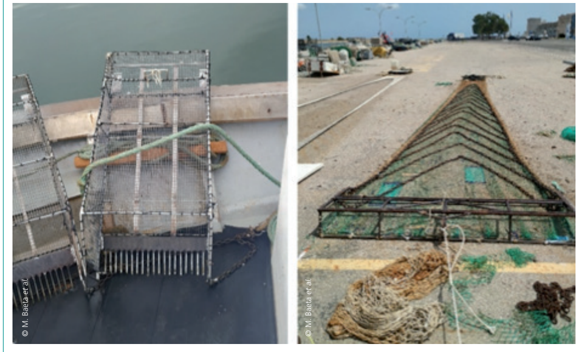
PLATE 32 Clam dredges used by mechanized clam dredge fisheries (left) and by towed dredge fisheries (right) in the Ebro Delta
