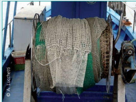
Square-mesh codend stored on a winch.
