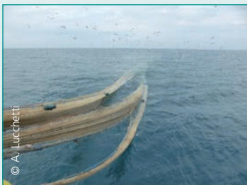
Trawl wing made of polyamide netting divided into an upper and a lower section (cut-wings).
