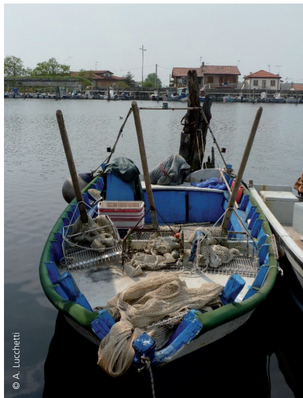
PLATE 46 Hand dredges operated from a vessel in Italy
