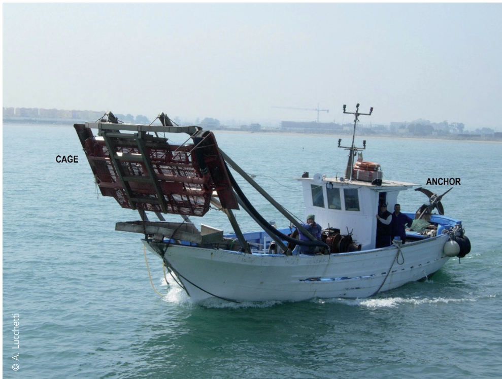
PLATE 43 Dredge (top) equipped with an anchor (bottom) for towing the cage
