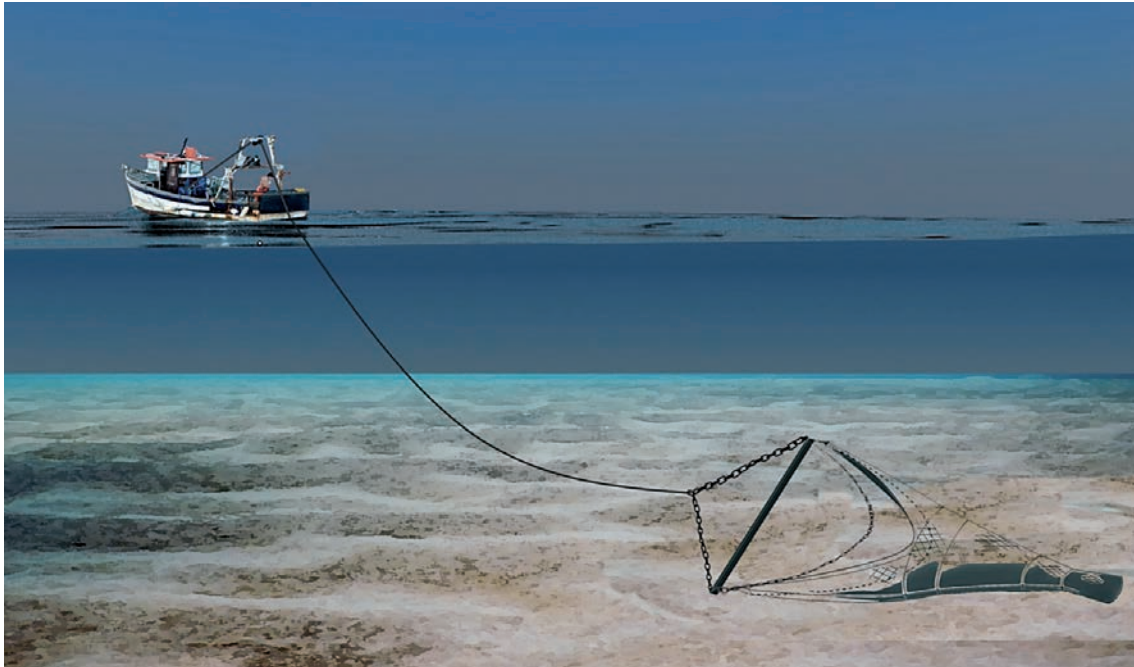
FIGURE 52 Drague barre dredge used in France
