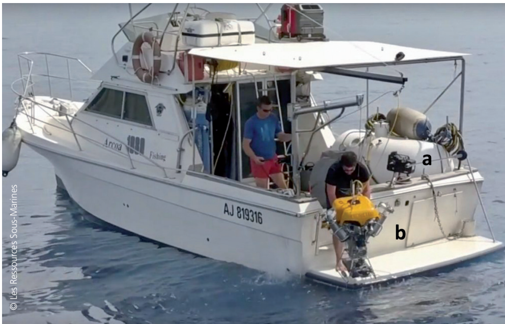
PLATE 76 Modern fishing vessel used for underwater fishing with decompression chamber (a) and remotely operated vehicle for prospection (b)
