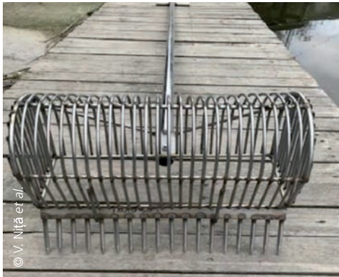
PLATE 48 Hand dredges being tested on the Romanian Black Sea coast to harvest bivalve species
