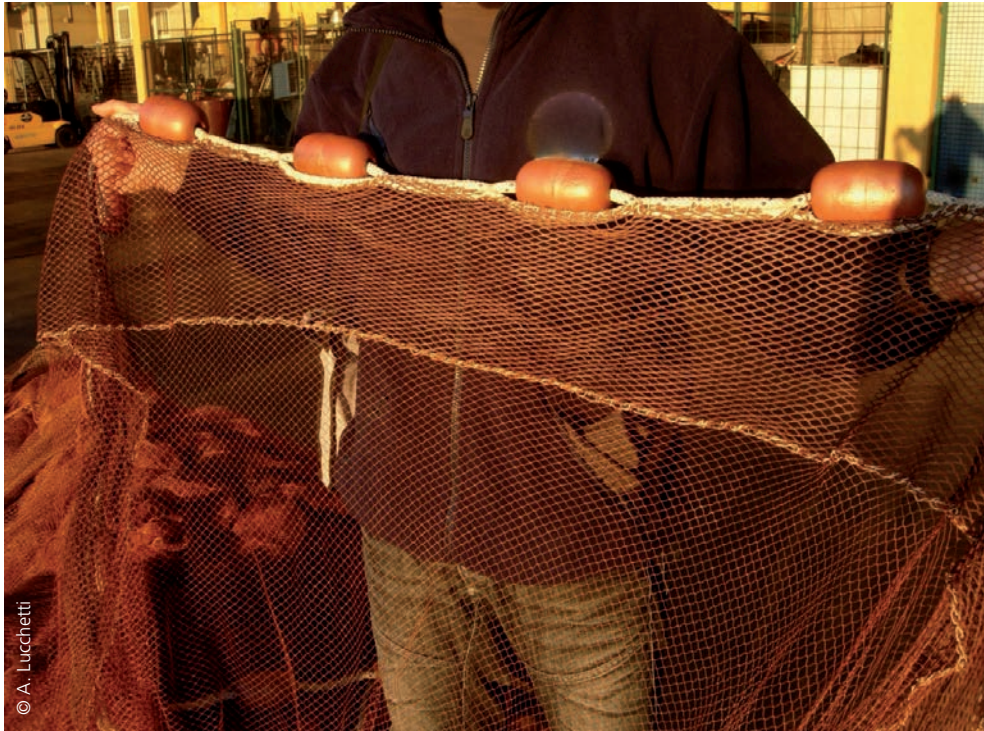
PLATE 21 Rigging of a purse seine for small pelagic species with reinforcement nets mounted on the headline and leadline
