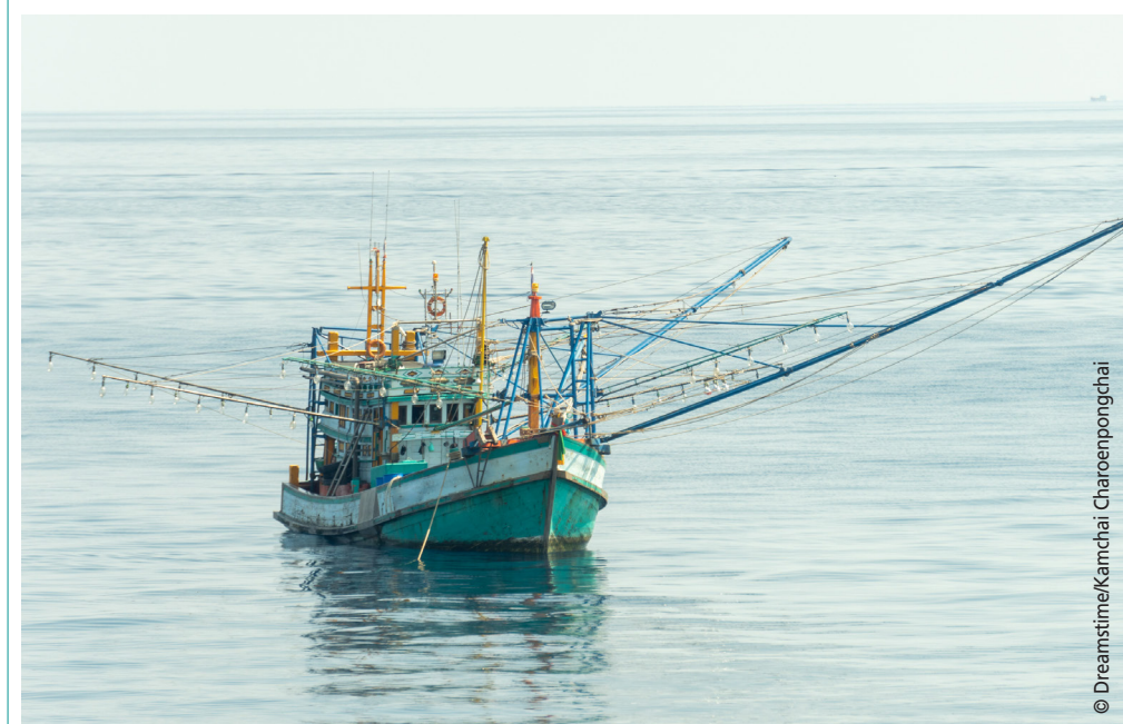
FIGURE 22 Lift netter operating
