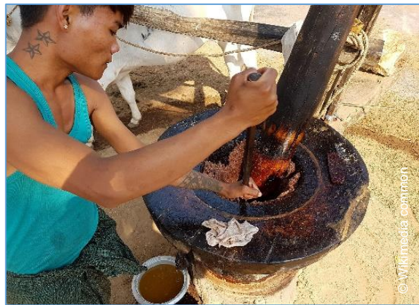
Figure 2. Extracting sesame oil by a bullock driven wooden pressing in Myanmar
