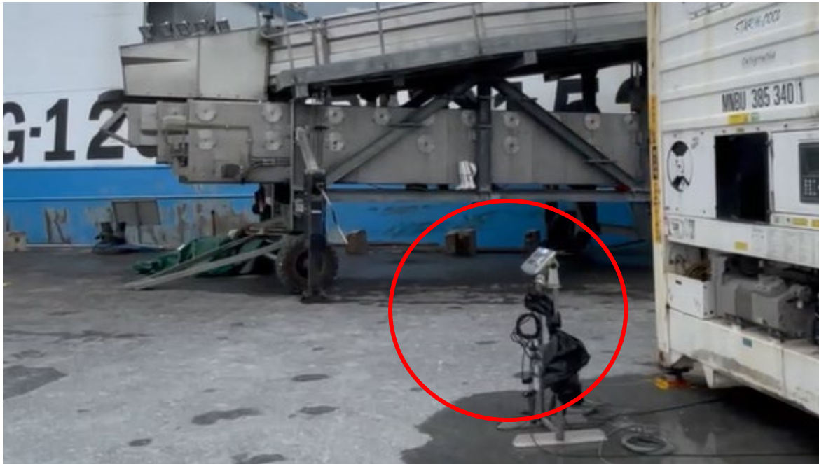
FIGURE 17: LOAD CELL USED TO WEIGH CONTAINER DURING LOADING TO MONITOR LOADING WEIGHT
