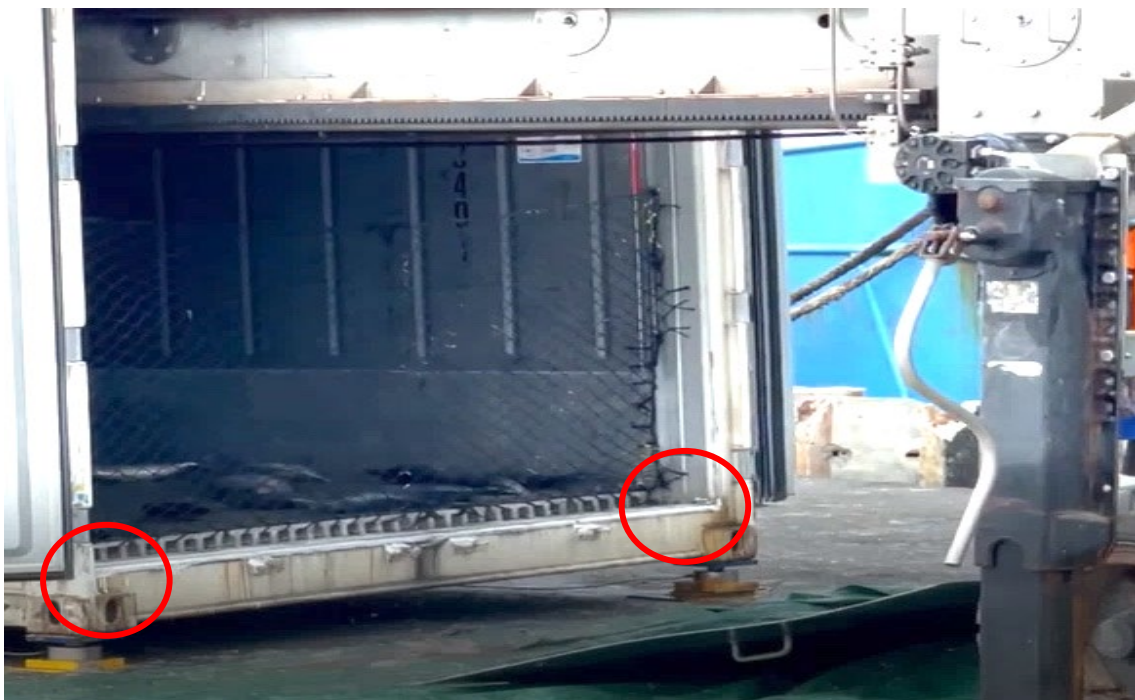
FIGURE 18: LOAD CELLS BEING USED DURING CONTAINER STUFFING
