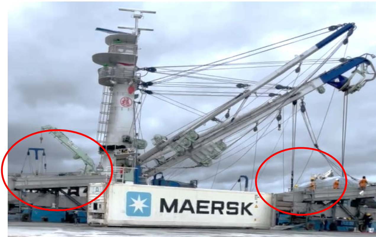
FIGURE 22: TWO STAR LOADERS SET UP READY FOR UNLOADING TWO HATCHES ON LARGER VESSELS
