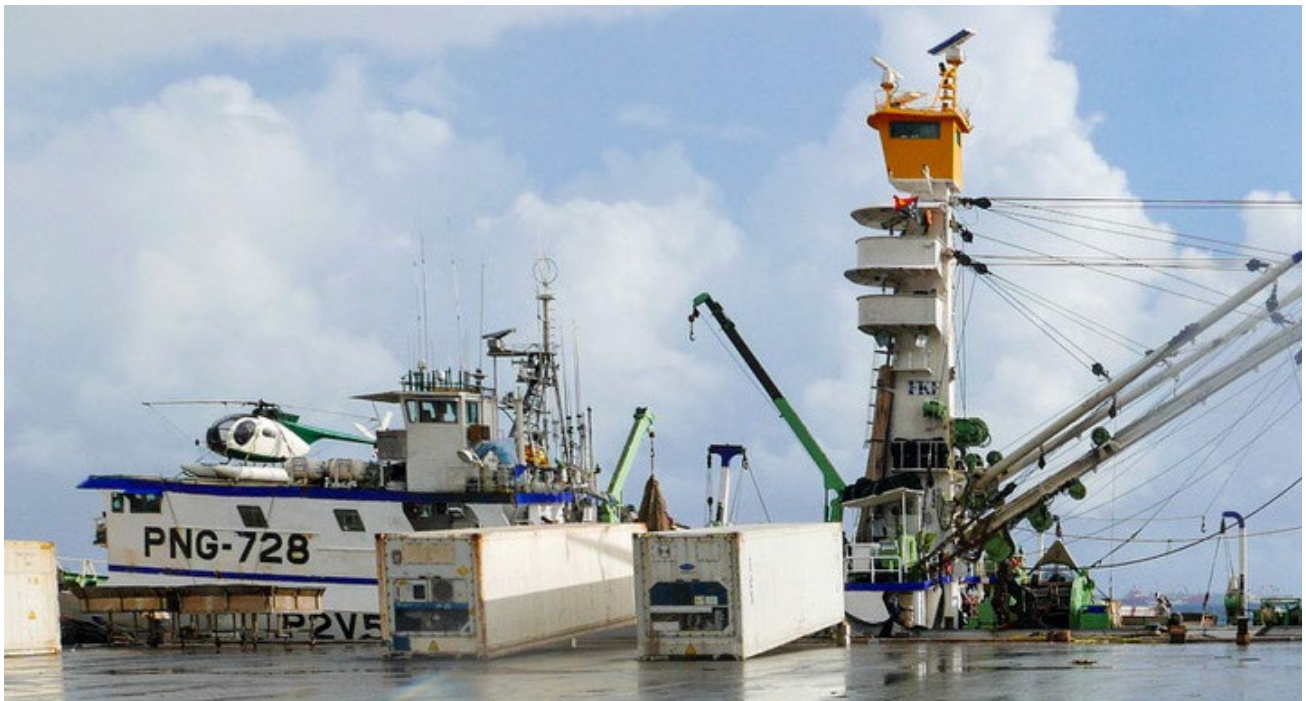
FIGURE 4. CONTAINERISATION FROM A PURSE SEINER IN WHARF WITH SPECIES SEPARATION TO EACH CONTAINER
