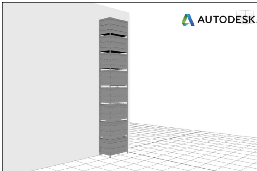
Figure 12. Eight bins stacked lengthways against the long wall of a cold room, parallel to the isle store 4mt of tuna
