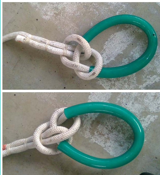
FIGURE 8.11 Extremity of the mooring line where the headline will be tied
