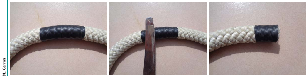
FIGURE 8.6 Cutting small diameter ropes
