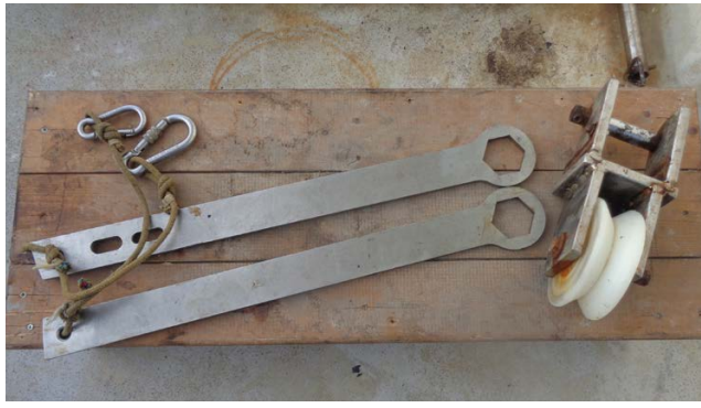
FIGURE 8.13 Wrenches and pulleys used when installing a mooring line
