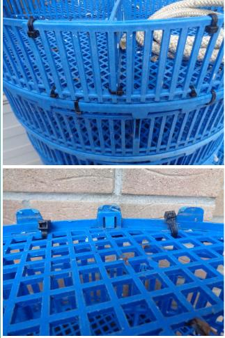
Conversely, for the structural integrity of the devices constructed with hard plastic mesh, repairs can be easily executed using heavy-duty cable ties (Figure 8.42).
