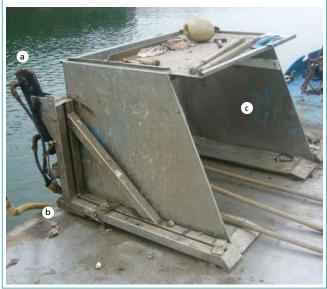
the ability to control the density of distribution and avoid any large clumps of oysters on the seabed. Depending on how the hydraulic system is set up, this can either be controlled by a crew member on deck or by the skipper in the wheelhouse.
