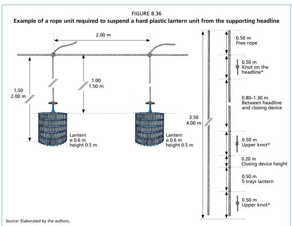
The distance between the headline and the top of the lantern will be 0.8–1.3 m, plus an additional 0.2 m accounting for the length of the lantern locking device (Figure 8.36).
