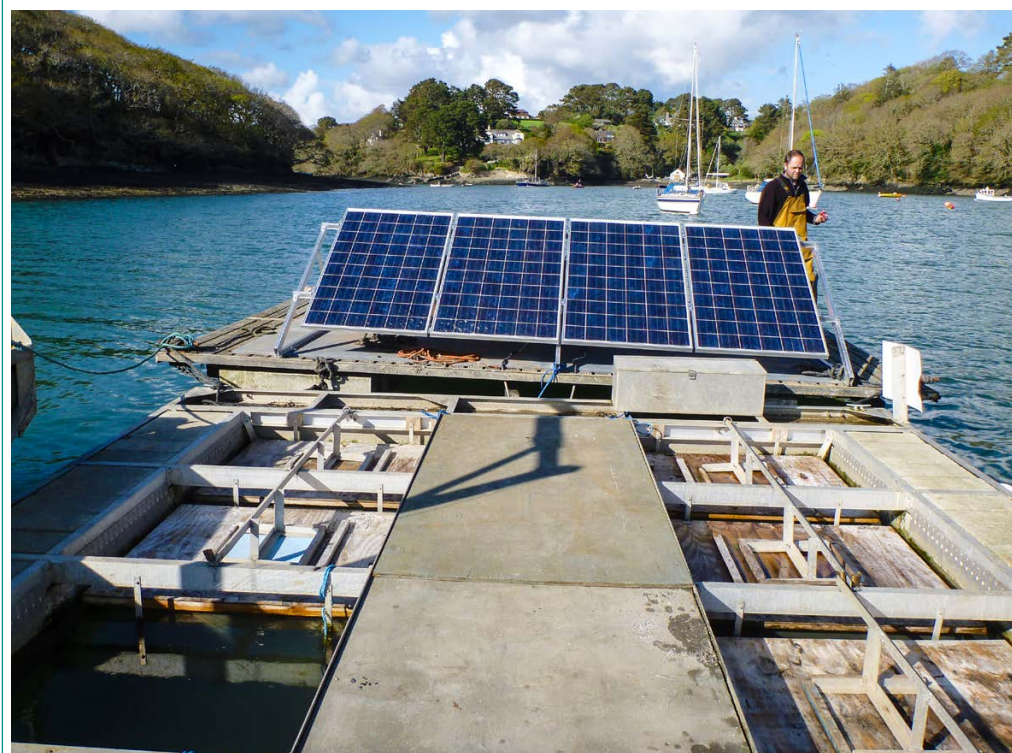
FIGURE 5.1 Upwelling raft powered by solar panels
