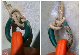
FIGURE 8.8 Knot used to secure an intermediate surface buoy Visible the security knot to prevent the rope from becoming dislodged
