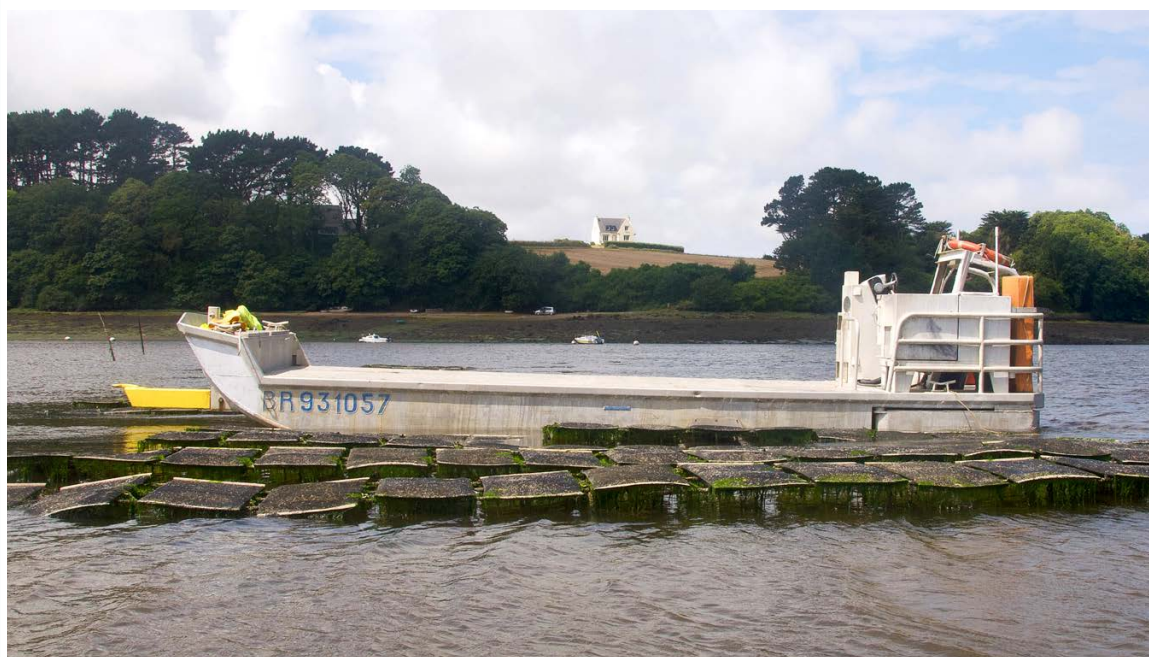
FIGURE 6.17 Oyster workboat next to trestles at Beg Ar Vill oyster farm, France. Note the shallow draft to allow access to the site in the minimum depth of water
