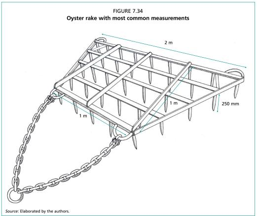
Another important role of the rake is to remove any excessive amounts of macroalgae. Small amounts of seaweed on the oyster beds will not cause any harm but, if significant quantities build up over the oysters, it can inhibit their ability to filter, slowing growth and, in extreme cases, cause mortality. When undertaking this task, the rakes must be hauled back on deck on a regular basis in order to clear the weed from the metal spikes.
