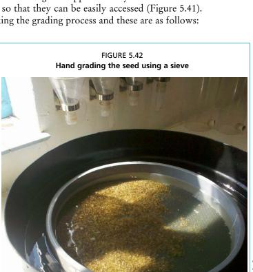
• The downgrade that has fallen through the mesh collects at the bottom of the tub. When the tub is full, it is drained of water and the smaller oysters are then tipped back into a seed box to be placed back on the Flupsy to allow them to develop further.
