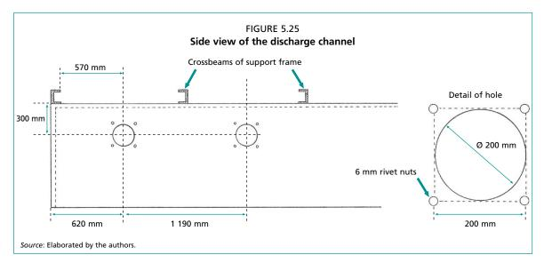
The flanges that are used to connect the seed boxes to the discharge channel are identical to the porthole sock supports that are mounted inside the seed boxes. Please reference page 111 and Figures 5.36c and 5.36d for further details. These should be attached using  $20 \times 6$  mm stainless steel bolts to the exterior of the discharge channel around the pre-cut 200 mm holes shown in Figure 5.25. There are 10 units in total.
