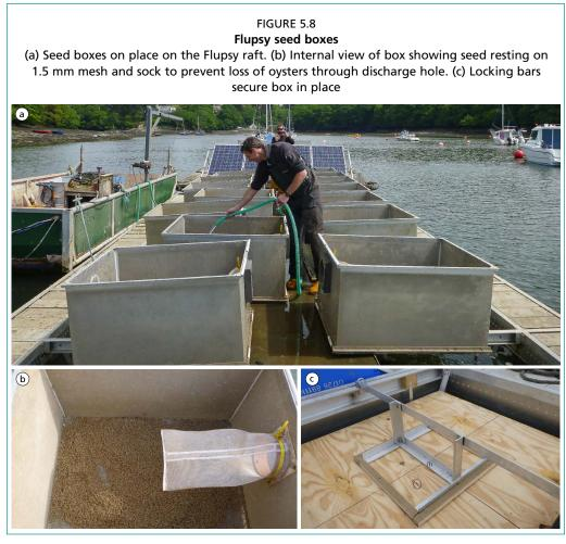
from 1.5 mm mesh stretched and glued over an aluminium frame. The box lids are made from marine ply and feature an inspection hatch for easy access to the oyster seed. The boxes are held in place by a locking bar made from aluminium angle. Not only does this ensure that the box remains lined up with the porthole in the discharge channel, but it also provides some security by limiting access to the seed.
