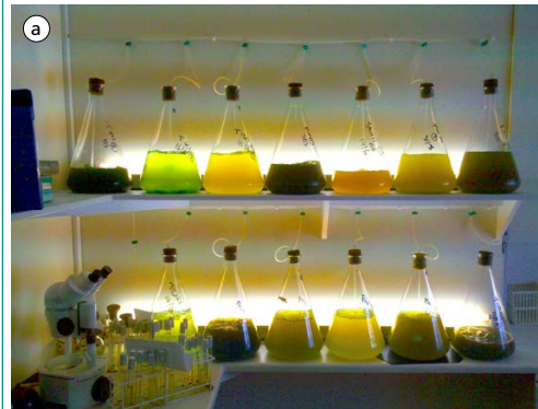
FIGURE 4.9 Algal cultures being produced at hatchery and nursery facility (a) Algal cultures produced using artificial UV light in flasks. (b–c) Algal cultures produced using artificial UV light in carboys and large plastic bags; and (d) Algal cultures produced outside using natural daylight (Morecambe Bay Oysters)
