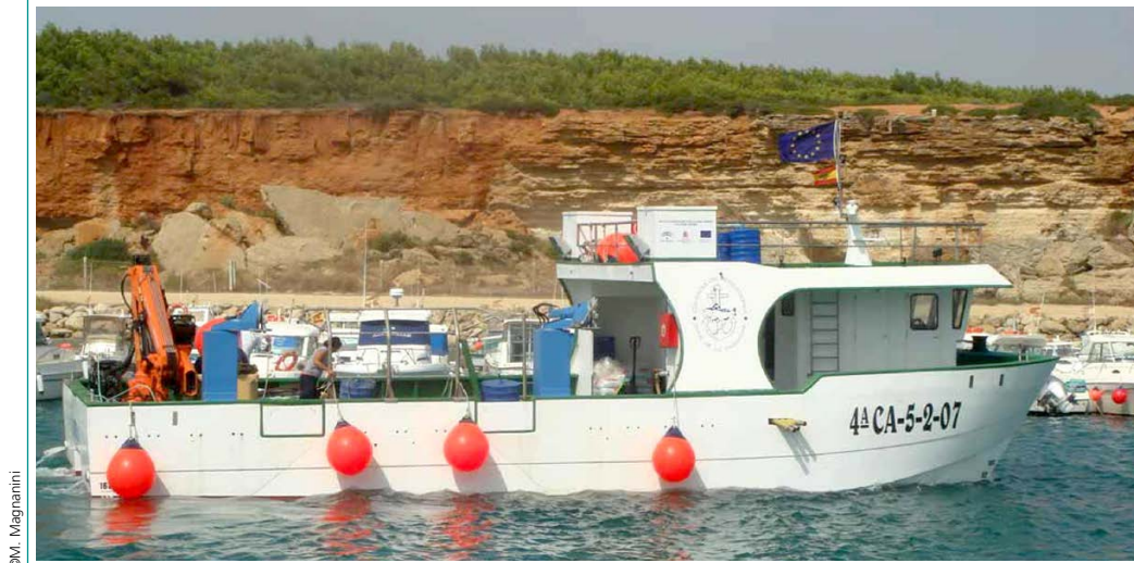
FIGURE 8.32 A bivalve long-line workboat equipped with a stern-mounted crane
