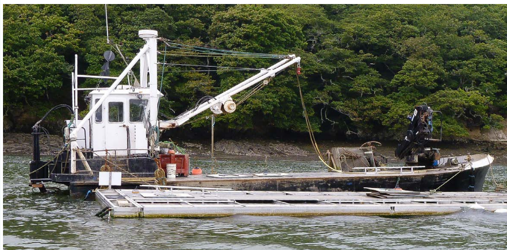
FIGURE 7.14 Examples of small oyster workboats with shallow draft and open deck space
