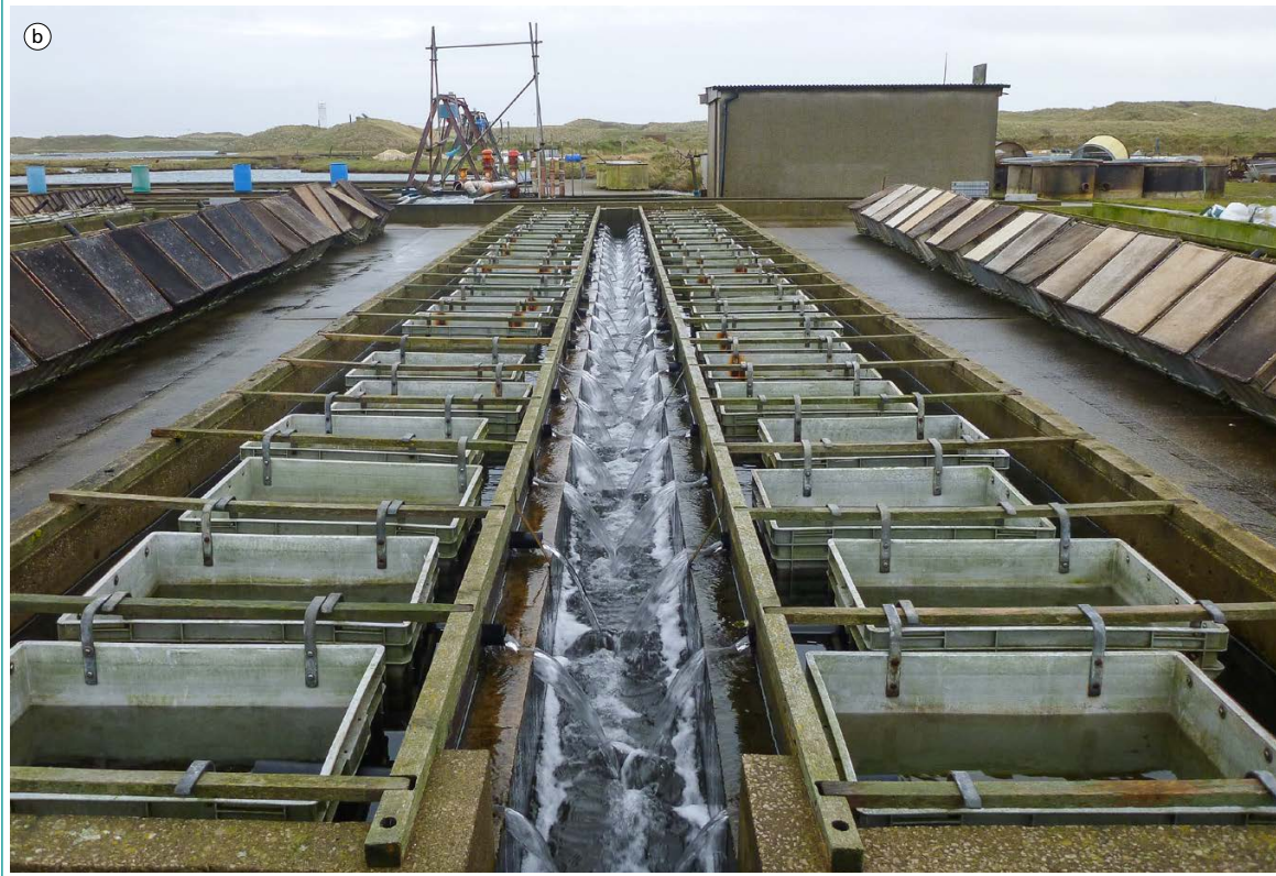
FIGURE 4.11 (b) Morecambe Bay Oysters hatchery and nursery facilities (b) Outdoor upwelling system fed by phytoplankton from the surrounding ponds
