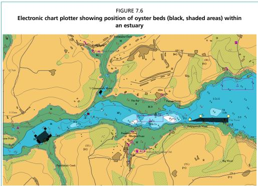
systems will show a "Track", which is an electronically generated line on the chart plotter indicating exactly which course the boat has taken when moving over the oyster beds. The skipper can refer to these "Tracks" to ensure that no ground has been missed and therefore minimise the oysters left behind after dredging.
