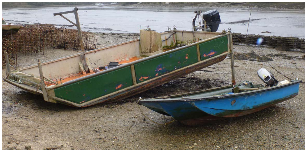
FIGURE 7.14 Examples of small oyster workboats with shallow draft and open deck space
