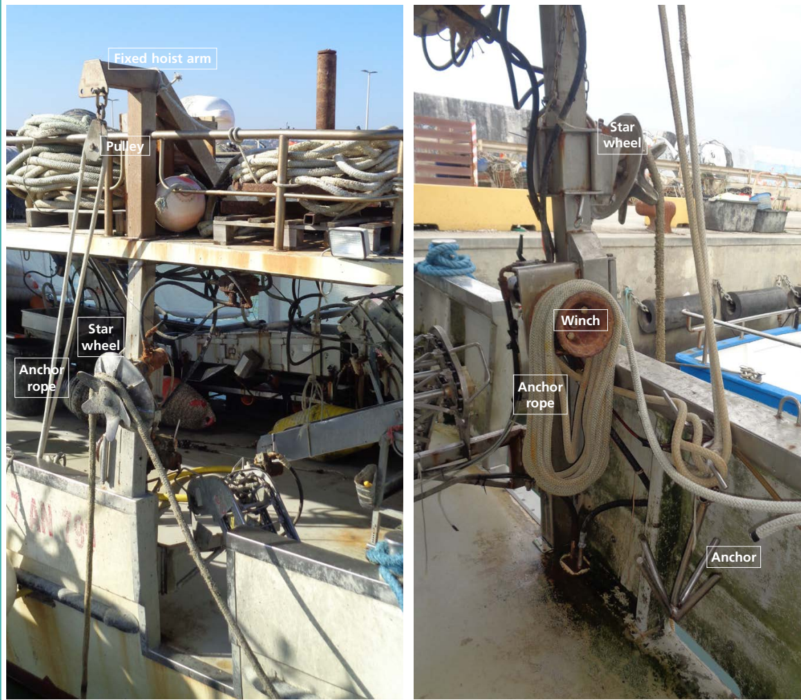
FIGURE 8.29 Images of the headline lifting device positioned at the stern of the workboat
