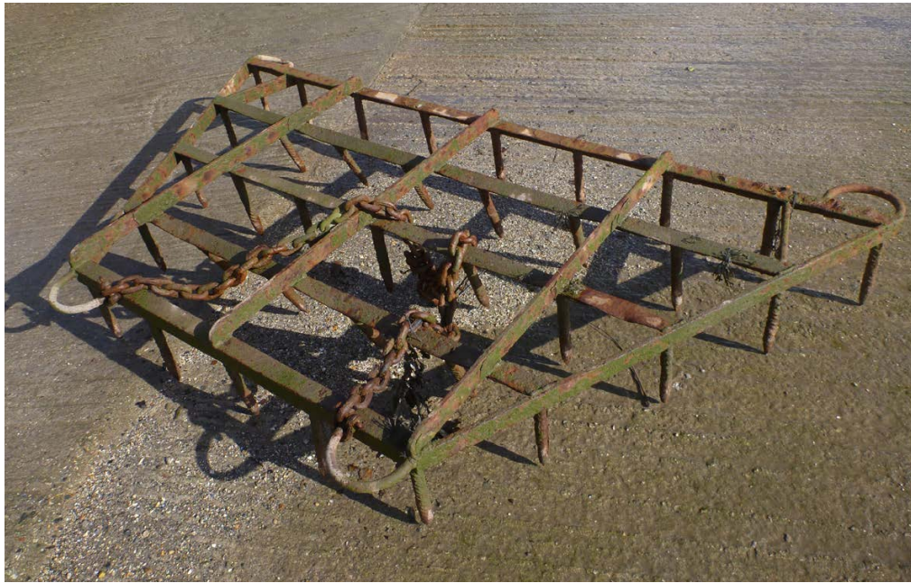
FIGURE 7.33 Oyster rake with rebar spikes configured in an offset pattern
