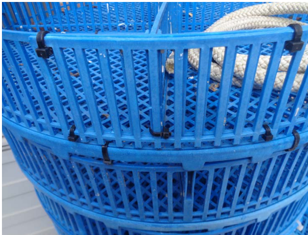
FIGURE 8.42 Repair of a hard plastic lantern
