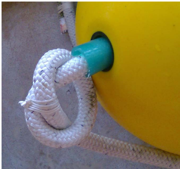
FIGURE 8.10 The knot employed on the upper side of the submersible buoy serving to secure the position of the buoy along the mooring line
