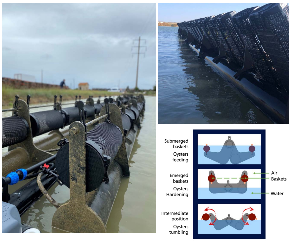
FIGURE 4.24 Example automated floating units with blower system
