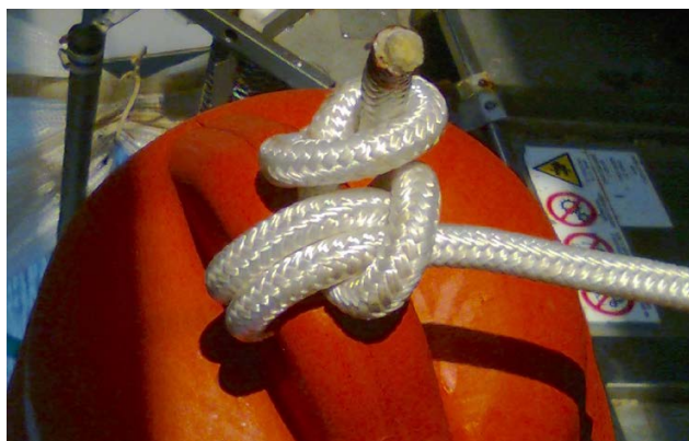
FIGURE 8.8 Knot used to secure an intermediate surface buoy Visible the security knot to prevent the rope from becoming dislodged
