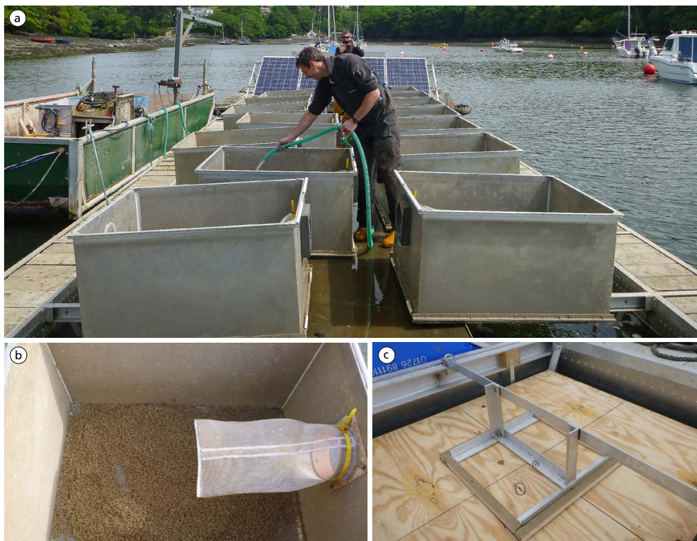
FIGURE 5.8 Flupsy seed boxes (a) Seed boxes on place on the Flupsy raft. (b) Internal view of box showing seed resting on 1.5 mm mesh and sock to prevent loss of oysters through discharge hole. (c) Locking bars secure box in place
