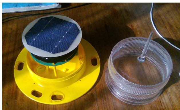
FIGURE 8.16 Solar-powered LED warning light fitted on a marker-buoy
