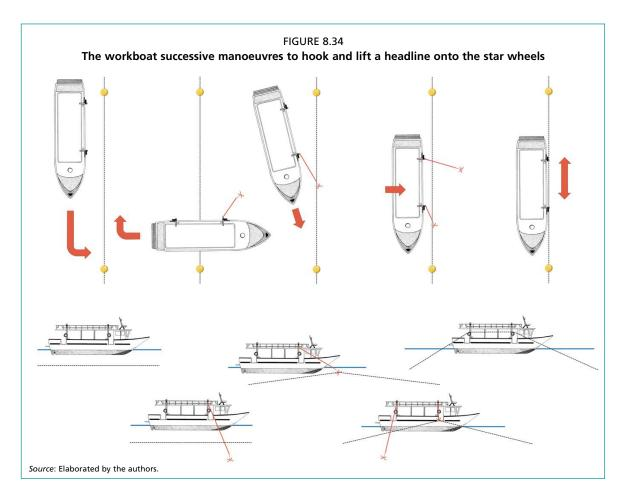
5) The second operator proceeds to manoeuvre the stern of the boat near the headline by pulling the rope of the stern anchor. At this point, with both anchors securing the headline suspended over their respective star wheels, the operators slowly release the winches simultaneously to facilitate the lowering of the headline onto the star wheels.
