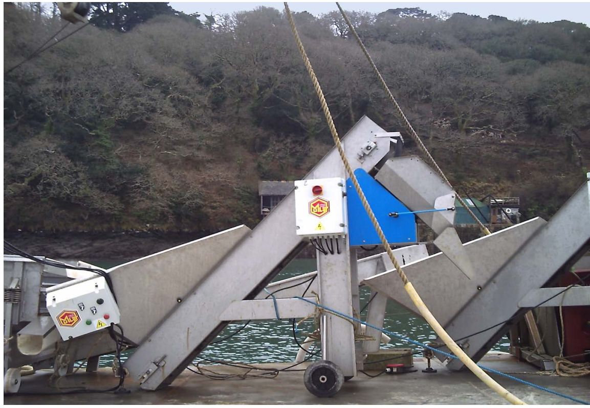
FIGURE 7.28 Shellfish weighing and bagging machines on deck
