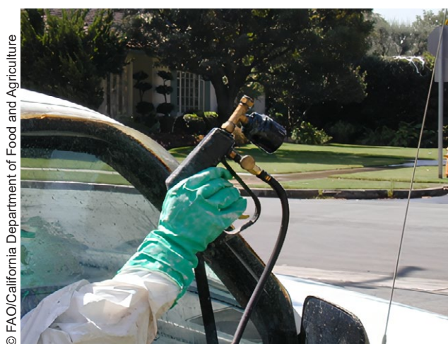
Figure 7.1. Application of MAT product using a high-pressure sprayer mounted on a truck
