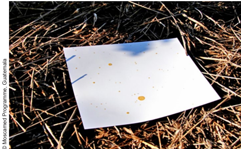
Figure 4.7. Kromekote cards (30 cm × 30 cm) showing the droplets of GF-120 after application of insecticide-bait by helicopter
