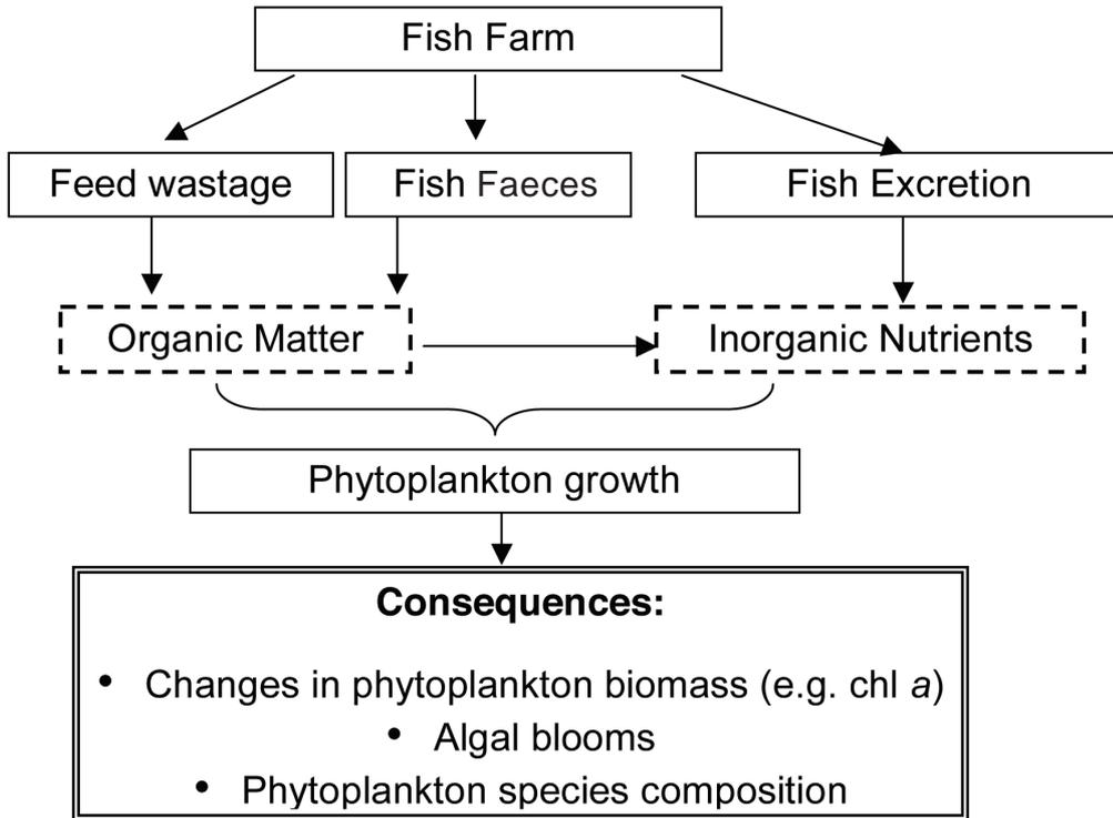
Figure 6.6.2 : Pathways of nutrients by fish farm operations to phytoplankton in water column. Exposure of nutrients depends on hydrodynamics, stratification and sediment-water exchange.
