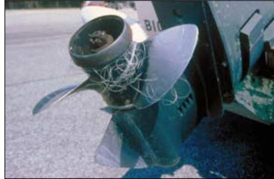
FIGURE 8 The effects of ALDFG on propellers
