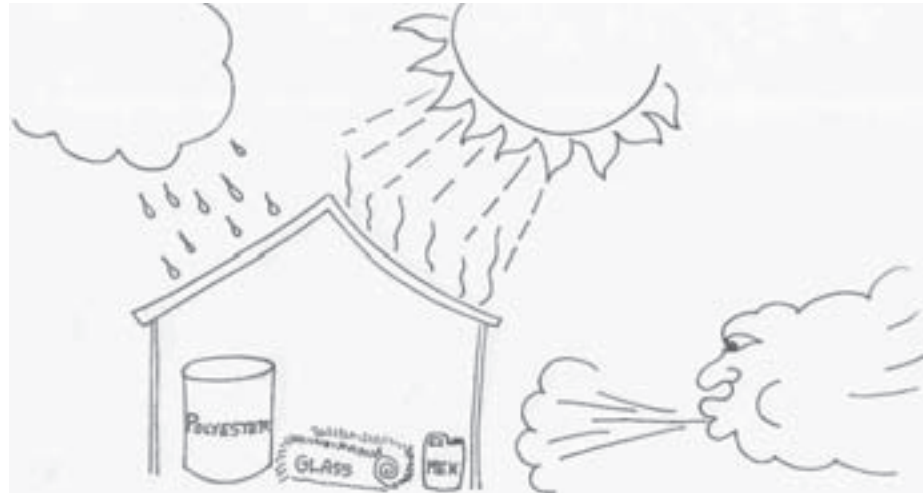
FIGURE 11 Storage of FRP materials
