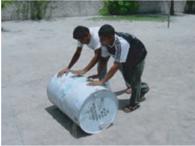
FIGURE 9 Mixing of resin
