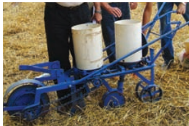
Plate 25 The Gralha azul animal traction no-till planter and fertilizer applicator developed at IAPAR in the mid-1980s
