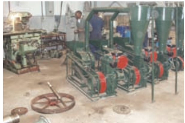
Plate 17 Hammer mill production in Nairobi, Kenya. (Making value-adding technology is attractive to manufacturers)
