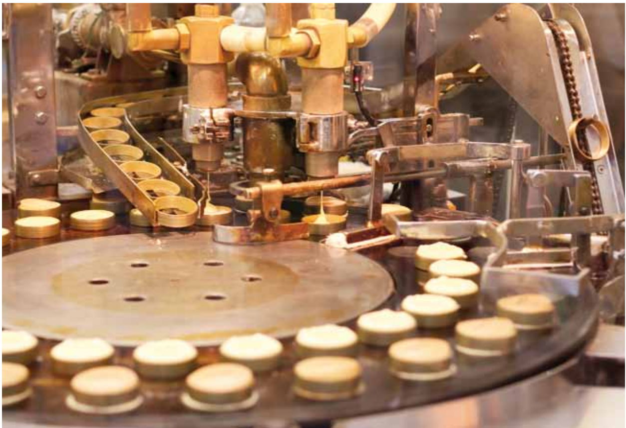
FIGURE 3. An array of half-cooked snacks, rotating for further processing
