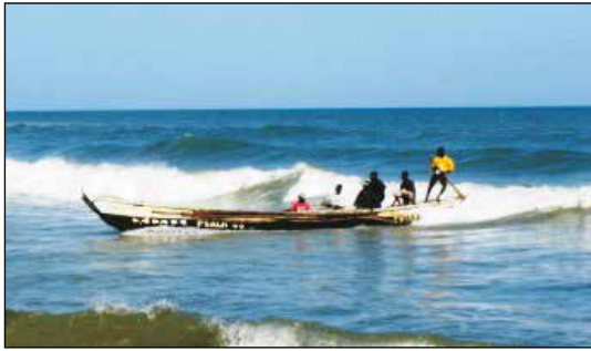
The canoes in Ghana are mostly operated from beaches with surf. The outboard engine of 25 to 40 hp is fitted on the side. Steering is done with a steering oar.
