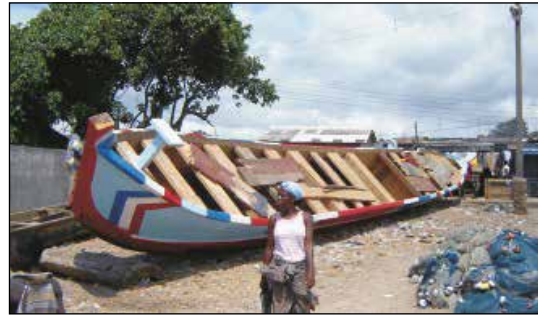
The canoes in Ghana are up to 19 m (60 ft) long. The bottom part is carved out of a single tree. The topsides are planked.
