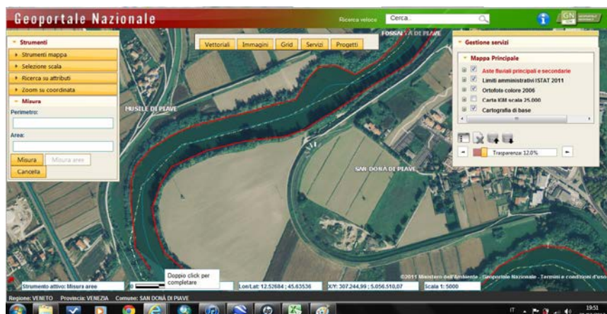
Figure IT.6. Example of section selected for the calculation of the area - National Geoportal.
