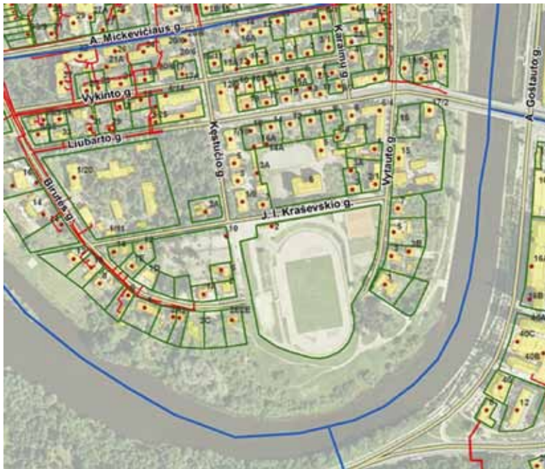
Figure 4 Extract from a GIS map showing parcel boundaries and centroids of buildings
