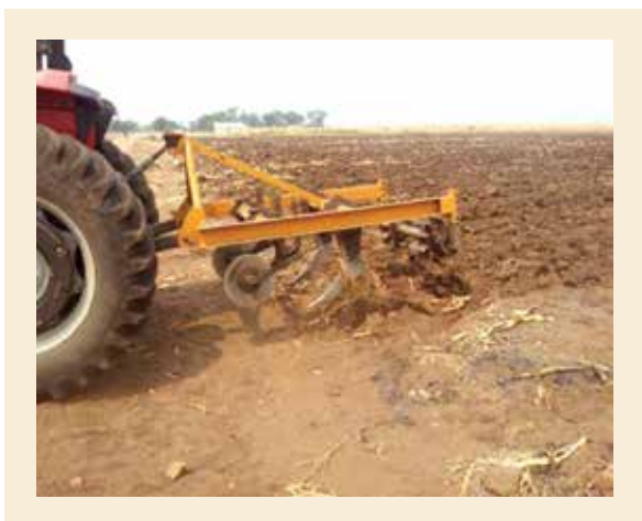
Ndume tractor ripper manufactured in Gilgil, Nakuru County, Kenya
