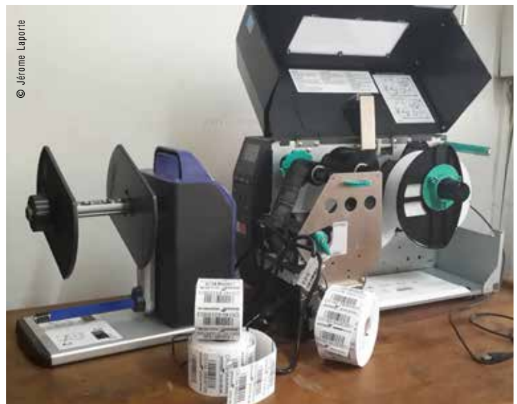
Photo 5 Printer and rewriter with newly printed labels
