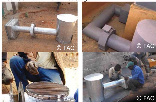
Image 7: FTT indirect smoke generator system
