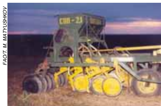
Plate 15 Direct seeder SZS-2.1 with cutting discs developed by the Shorthandy Institute
