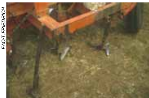
Plate 9 Original SZS-2.1 hoe-drill coulter
