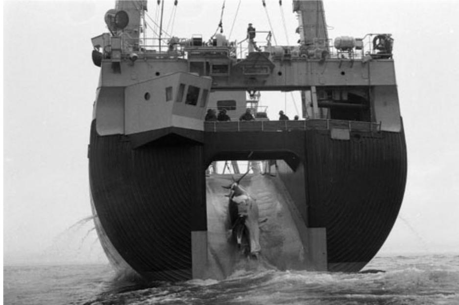
**The stern-ramp, typical of modern factory-ships, revolutionized pelagic whaling**
