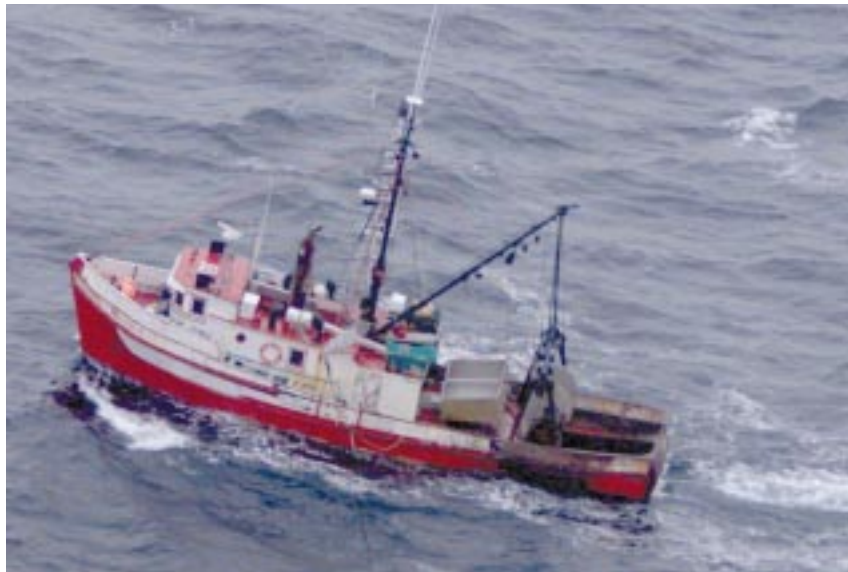
A typical 65' Scotian-Fundy 'dragger' that would have participated in the mobile gear ITQ programme
