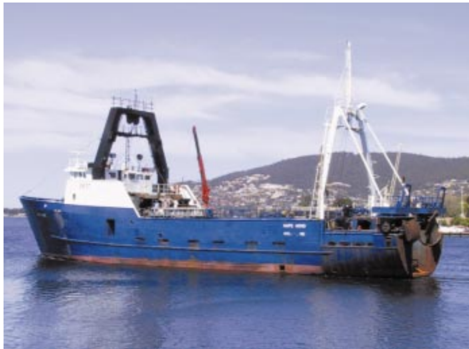
The Cape Hood , seen here undergoing engine trials in Hobart harbour, October 2001, is an example of vessels entering the orange roughy fishery off Tasmania. One of four in its class, she was built in 1975 in Pictou, Nova Scotia, for use in the Canadian northern cod fishery. The 45.9m, 2400 BHP, 189 GRT vessel was originally owned by H.B. Nickersons of North Sydney, N.S., Canada
