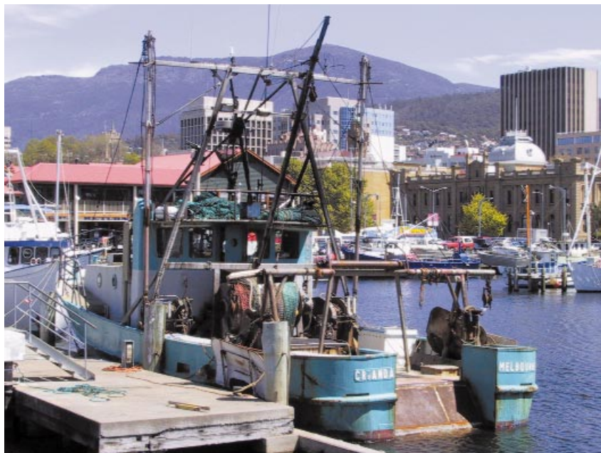
The Crianda , 18.2m LOA, 440hp, 60GT, shown above in Victoria Dock, Hobart, was completed in 1980 in Melbourne, Victoria. It is typical of the trawlers targeting “anything that swims” in the South East Fishery for market species.
