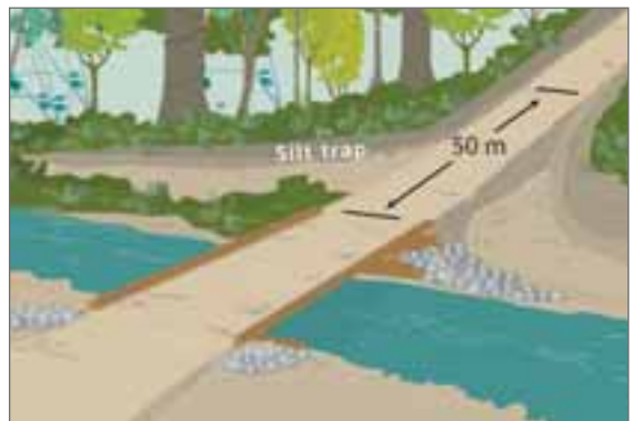
Figure 16 Correct siting of a bridge
