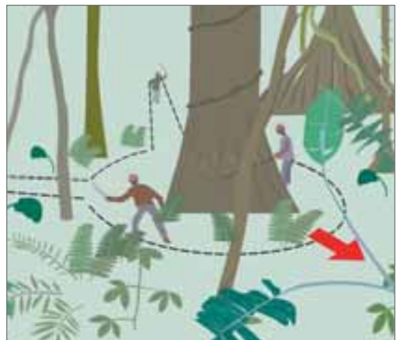
Figure 21 Escape routes and clearing around tree base
