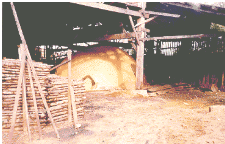
Figure 12: Brick Beehive Charcoal Kiln, HCMC
