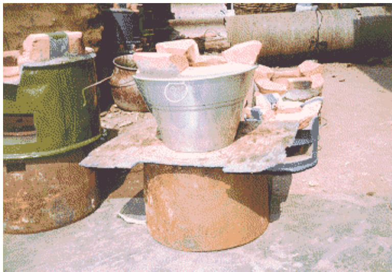
Figure 13: The Second, and the Smallest, Model of Improved Cookstove Introduced.
