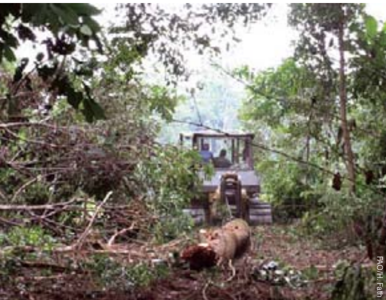
Environmentally friendly harvesting: skidding of Okume ties on a preplanned skid trail, without damage to soil or residual vegetation, Gabon
