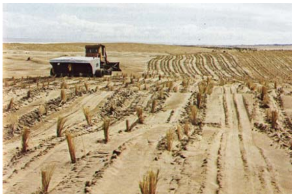
Plate VI A marram planting machine capable of planting 20 ha of marram grass per day
