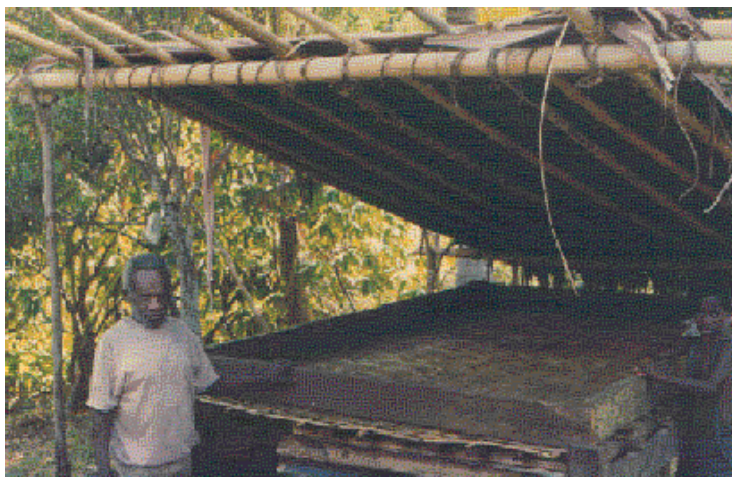
Figure 13. Small dual drier made from bush materials
