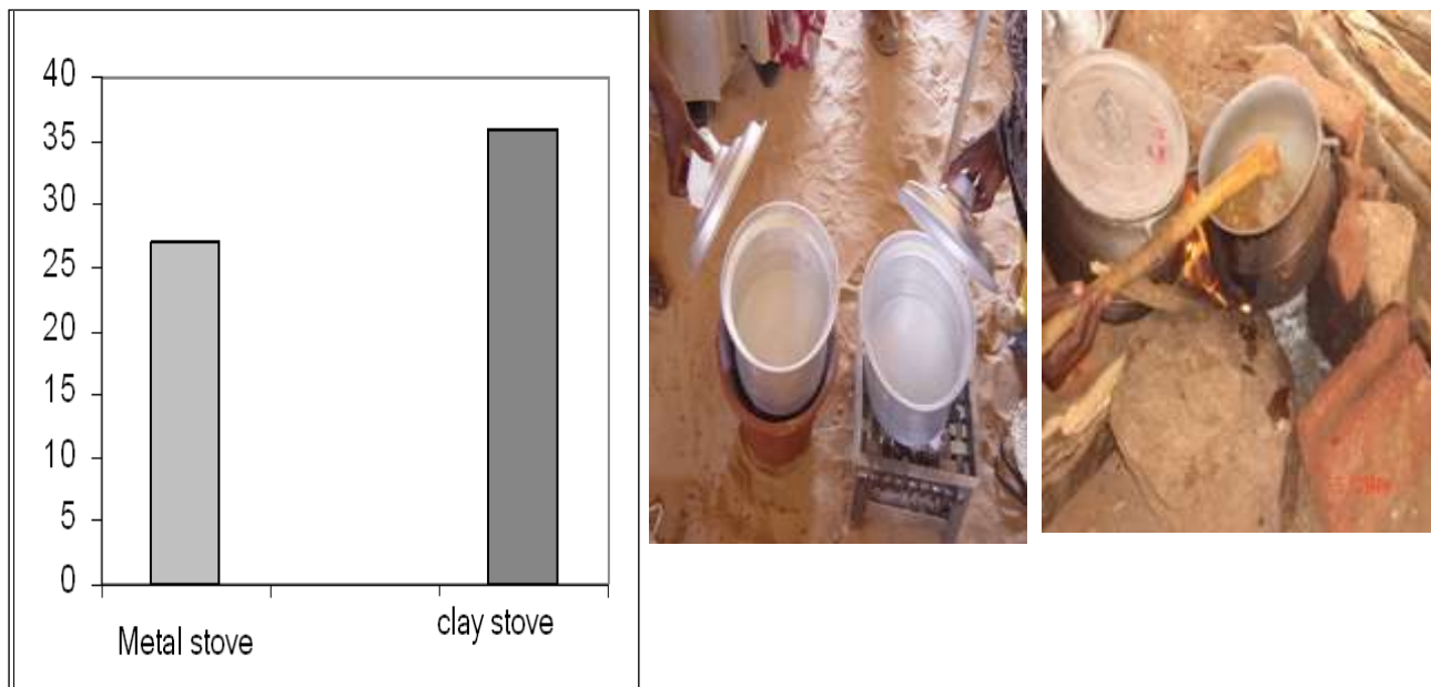
Figure 3. (right) Cooking stoves: traditional three-stones stove; (middle) traditional metal stove and improved clay stove "Kanoon Elsirur"; (left) bar chart showing levels of energy efficiency of the traditional metal and improved clay stoves. (Source: Practical Action 2008)
