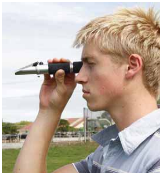
Assessing the sugar content (Brix) of pasture sap with a hand-held refractometer.
