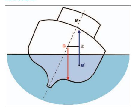
When heeled by an external force, the vessel's centre of gravity (G), which is unaffected by the heel and the weight (of the vessel), is considered to act vertically downward through G. The centre of buoyancy (G) (being the geometric centre of the underwater section) has moved to a new position G and the force of buoyancy (equal to the weight of water being displaced) is considered to act vertically up through the new centre of buoyancy G.
