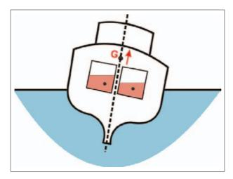
Partially-filled tanks have the greatest adverse effect upon a heeled vessel's metacentric height (GM). The division of the tank into two equal parts by the use of a watertight bulkhead will reduce the adverse effect on the vessel's metacentric height (GM) by up to 75 percent of that of an undivided tank.
