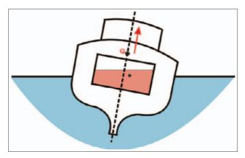
When a vessel with a partially-filled tank is heeled, the liquid will seek to remain parallel with the waterline. The centre of gravity of the liquid, being the centre of its volume, will move with the liquid and can have a considerable effect upon the vessel's stability. This effect is similar to that caused by adding weight on deck, i.e. rise of the vessel's centre of gravity (G) which causes a decrease in the vessel's metacentric height (GM) and thereby its stability.
