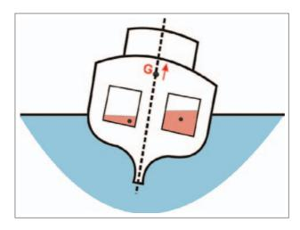
Care should be taken when endeavouring to correct a list by filling tanks. Having two partially-filled tanks will create additional free surface effect. If there is a possibility that the vessel's list is caused by loll, it is recommended that the tank on the low side be filled before commencing to fill the tank on the high side.
