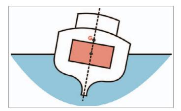
When a vessel with a full tank is heeled, the liquid within the tank acts like a solid mass. Its centre of gravity, being the centre of its volume, remains constant and therefore does not cause any change in the vessel's centre of gravity (G) or its metacentric height (GM) as the vessel is heeled.
