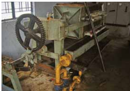
PLATE 17: Plate filter in a biodiesel production plant, India.
