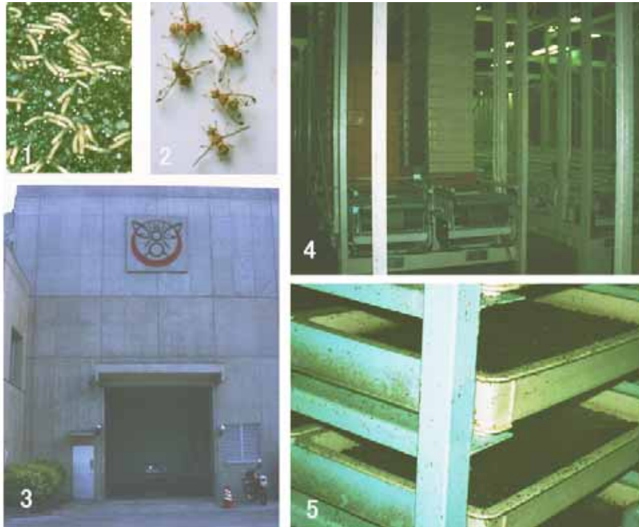
Plate 1. A plant producing sterile melon flies for their eradication: (1) larvae, (2) adults, (3) main building, (4) part of the automated rearing system, (5) feeding trays for larvae (Courtesy Jun Mitsuhashii)
