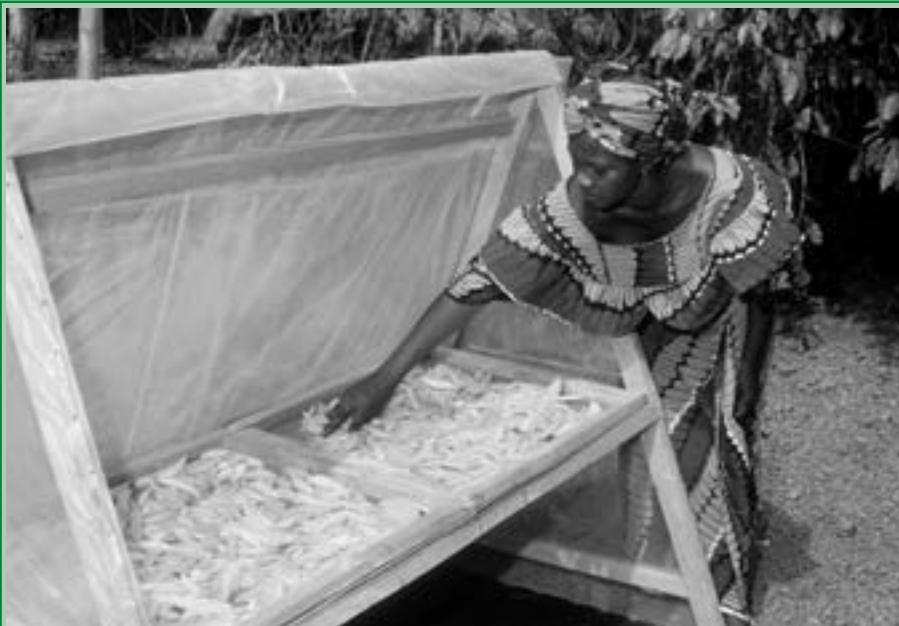
FIGURE 19 A simple solar dryer (Photo: FAO/15837/ R. Faidutti)
