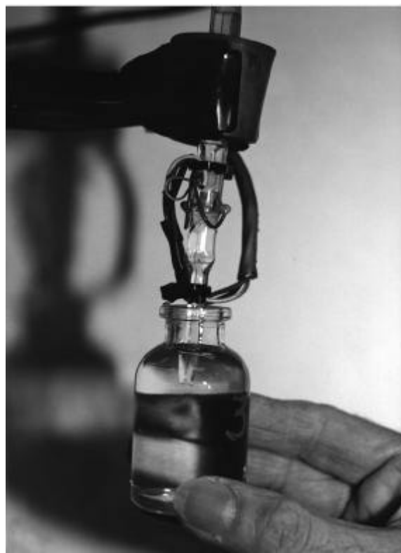
FIGURE 6 Measurement of the electrical conductivity of a saturated-paste extract ( EC_e ) using a laboratory micro-conductivity cell
