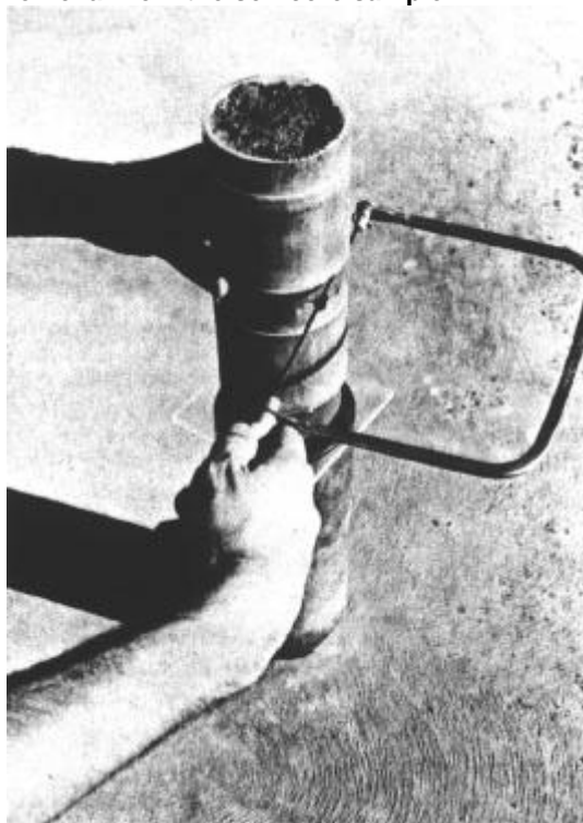
FIGURE 1.1 Series of four-electrode cells containing undisturbed soil-cores being segmented after removal from the soil-core sampler
