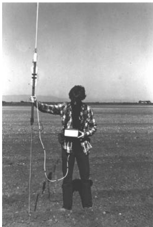
FIGURE 56 Antenna, battery pack and meter for measuring location on the landscape using the LORAN technique (after Rhoades et al. , 1990c)
