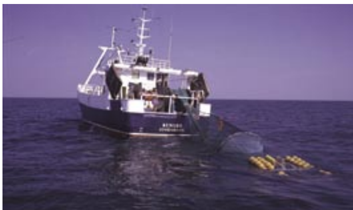
FIGURE 11 Setting out the trawl, codend cover and collection cage-unit from a trawler. The cover around the codend is supported by two hoops. The timers of the release-unit can be seen on the surface.
