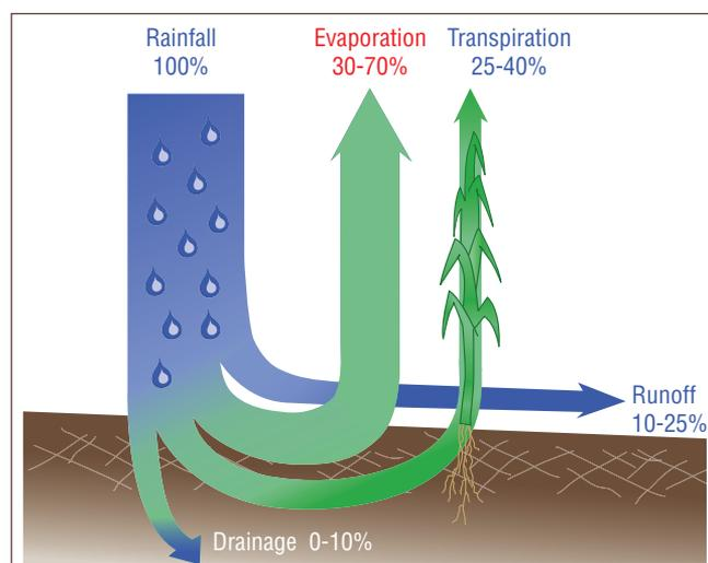
Figure 3: Productive water (transpiration) and water losses (evaporation and runoff) without water conserving measures in dry lands.
