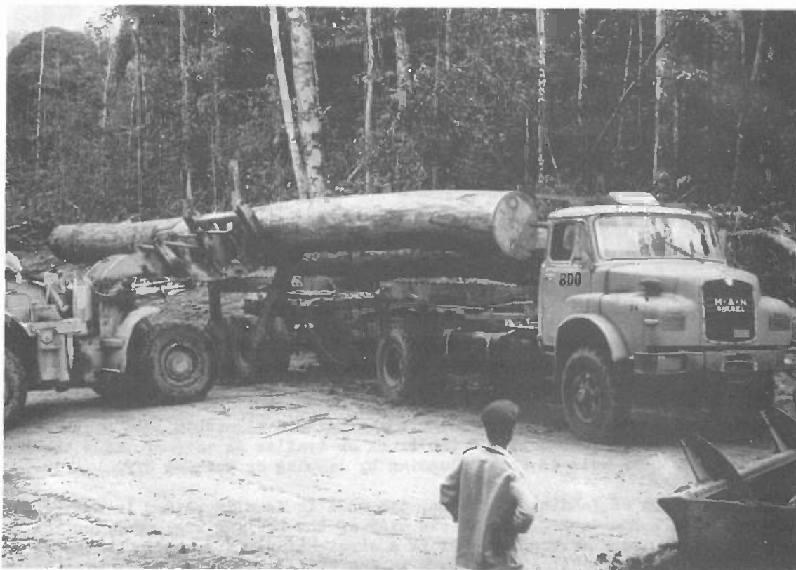
Truck loading by wheeled front end loader with log fork
