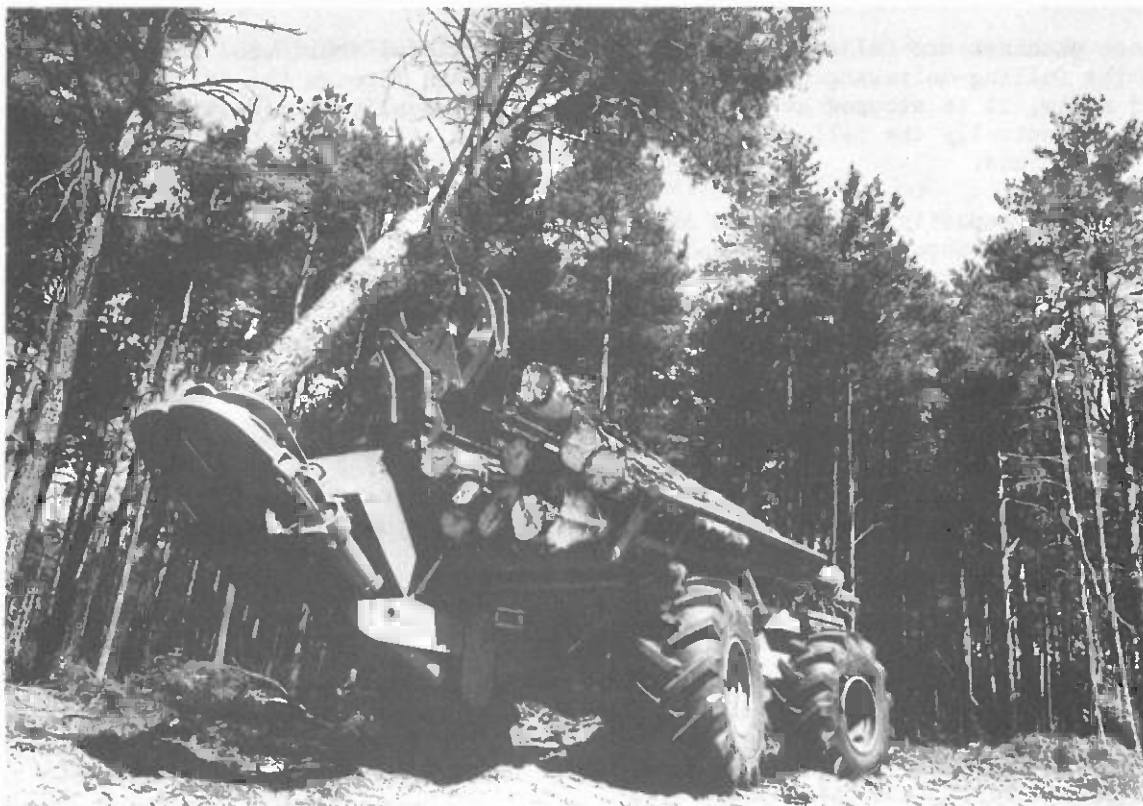
Feller-delimiter-forwarder laying down cut tree on rail-mounted delimbing carriage
