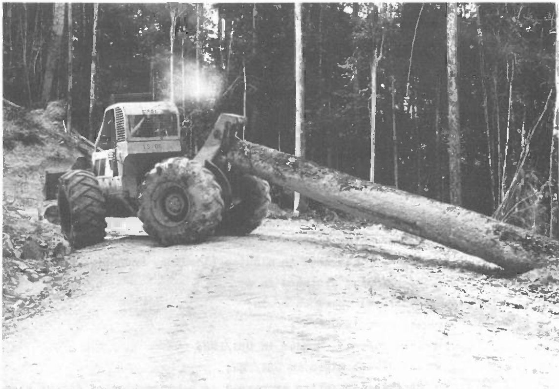
Wood extraction by skidder to the road
