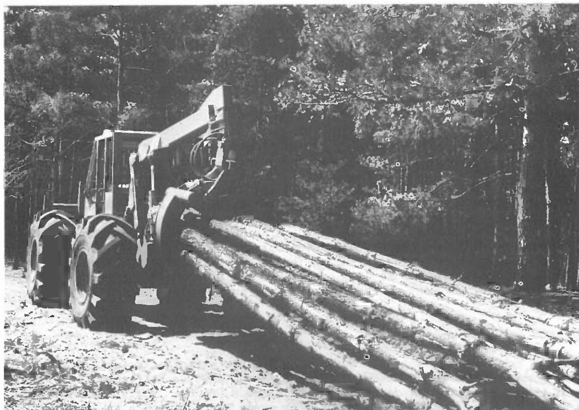
Grapple skidder extracting a load of logs
