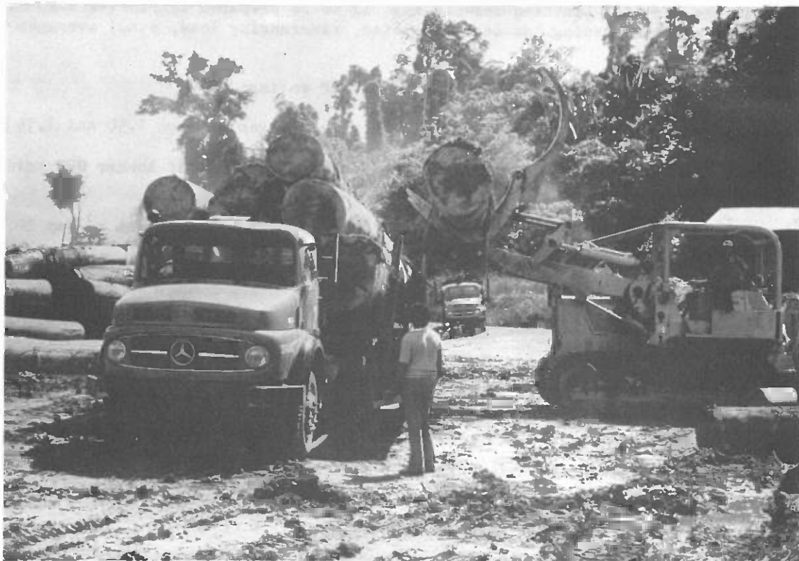
Crawler mounted front end loader unloading roundwood at the final landing
