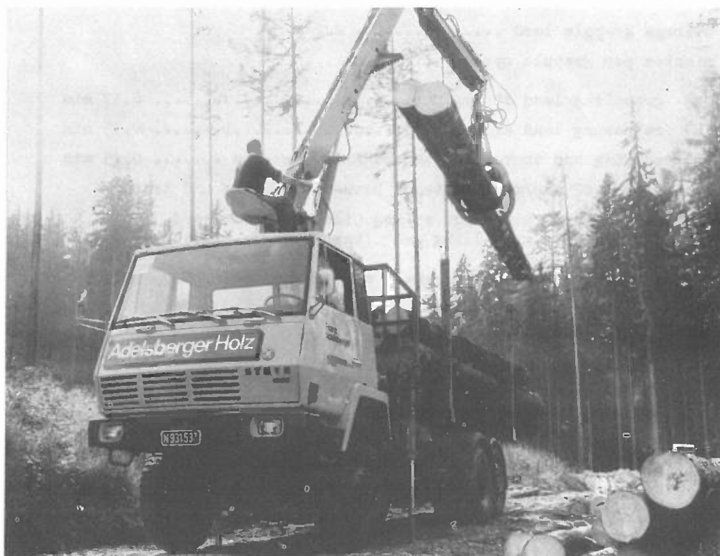
Truck mounted hydraulically operated loading crane
