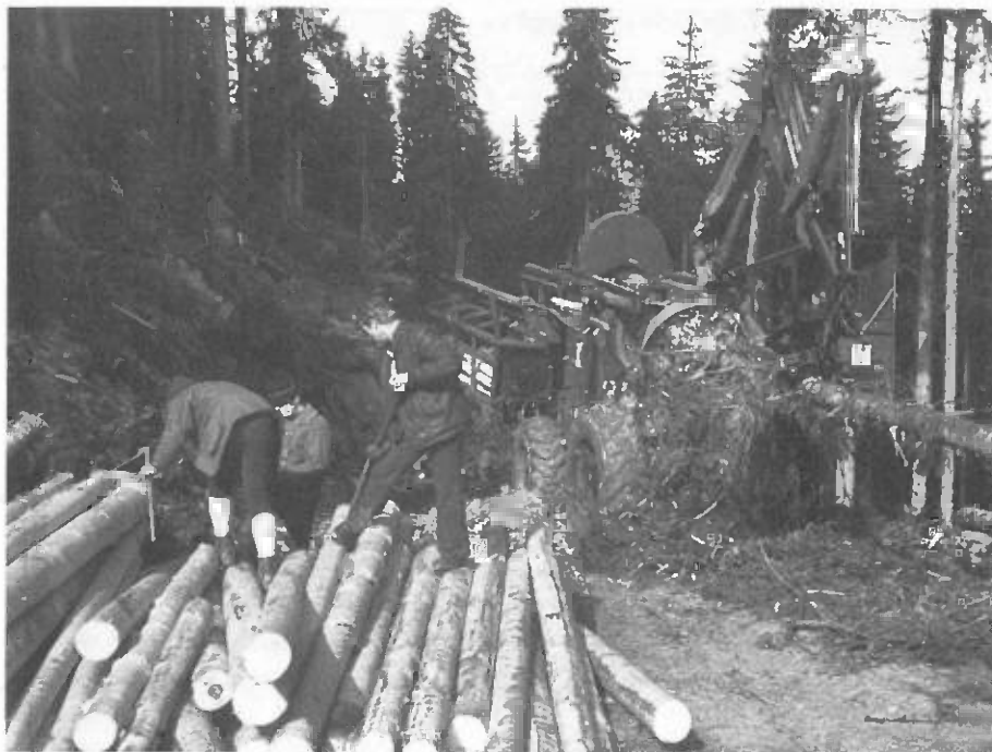
Processor picking up tree length logs for debranching, debarking, crosscutting and making assortments.
