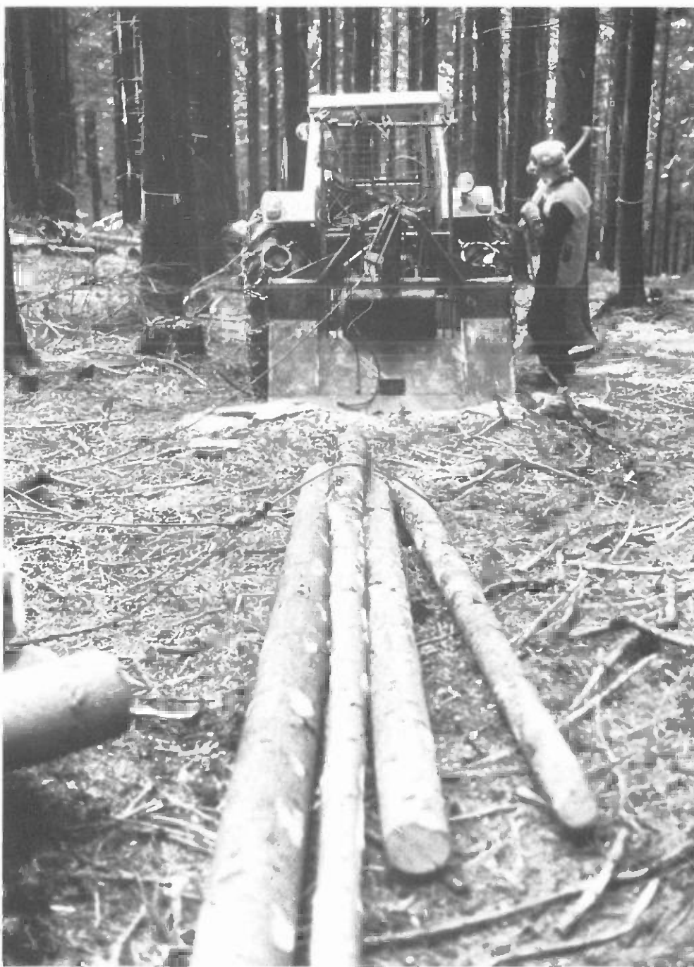
Tractor equipped for forestry work with heavy-duty tyre chains and integrally mounted skidding winch. Note cable mainline and chokers with quick-hitch couplings in foreground (Photo: R. Heinrich)
