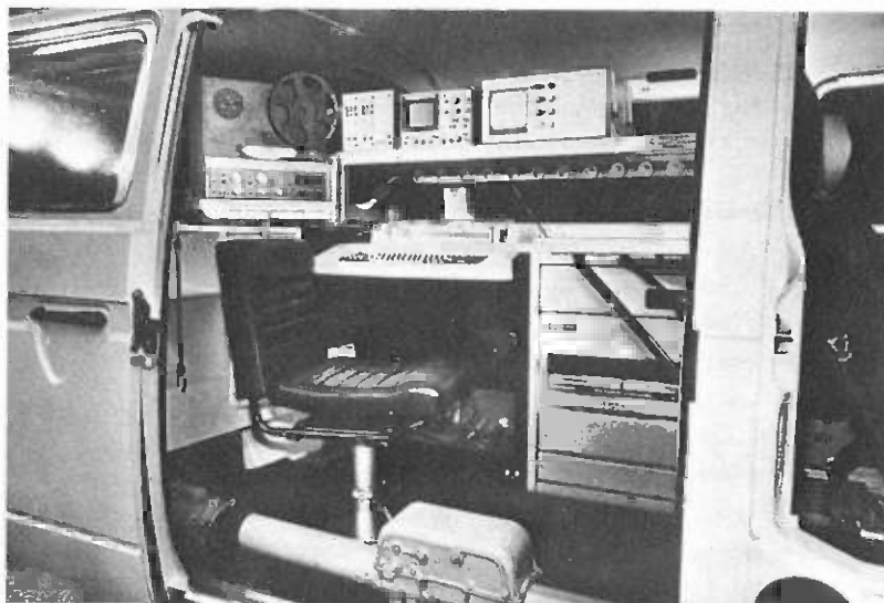
Mobile telemetric computer unit built into VW minibus
