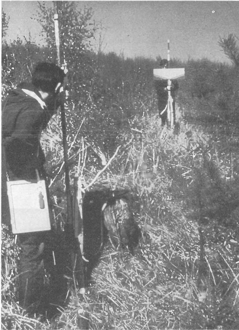
Surveying a forest road with a clinometer (Photo: E. Pestal)
