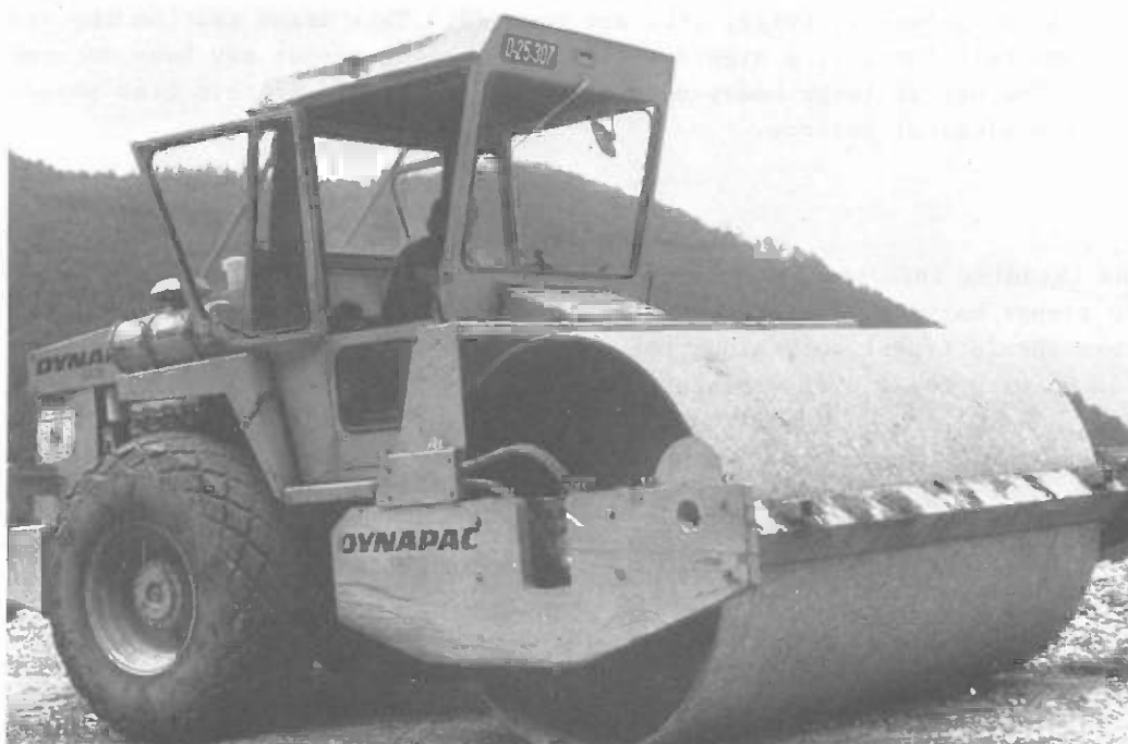
Dynapac roller often used for subgrade compaction in properly designed forest roads
