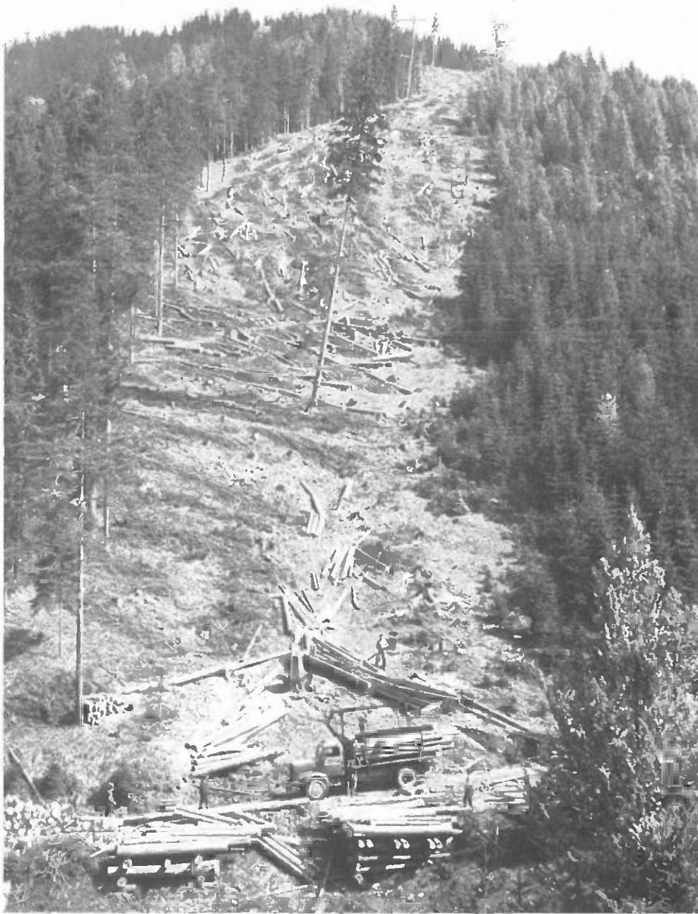
Strip clearcut, downhill log transport by cable crane. Truck being loaded by hydraulic loader. (Photo: Federal Forestry Research Institute)
