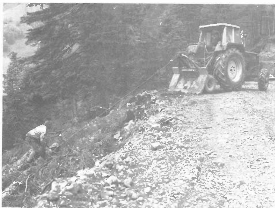
Farm tractor with bogie used for uphill ground skidding (Photo: Steyr)
