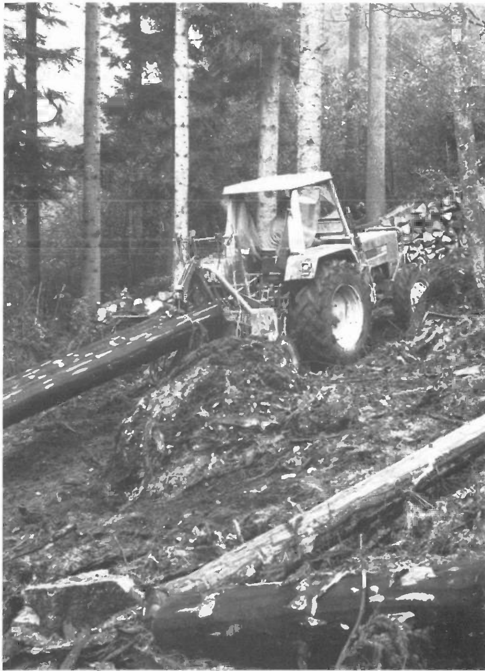
Steyr four-wheel-drive tractor with logging trolley being utilized to skid logs to roadside (Photo: Steyr)
