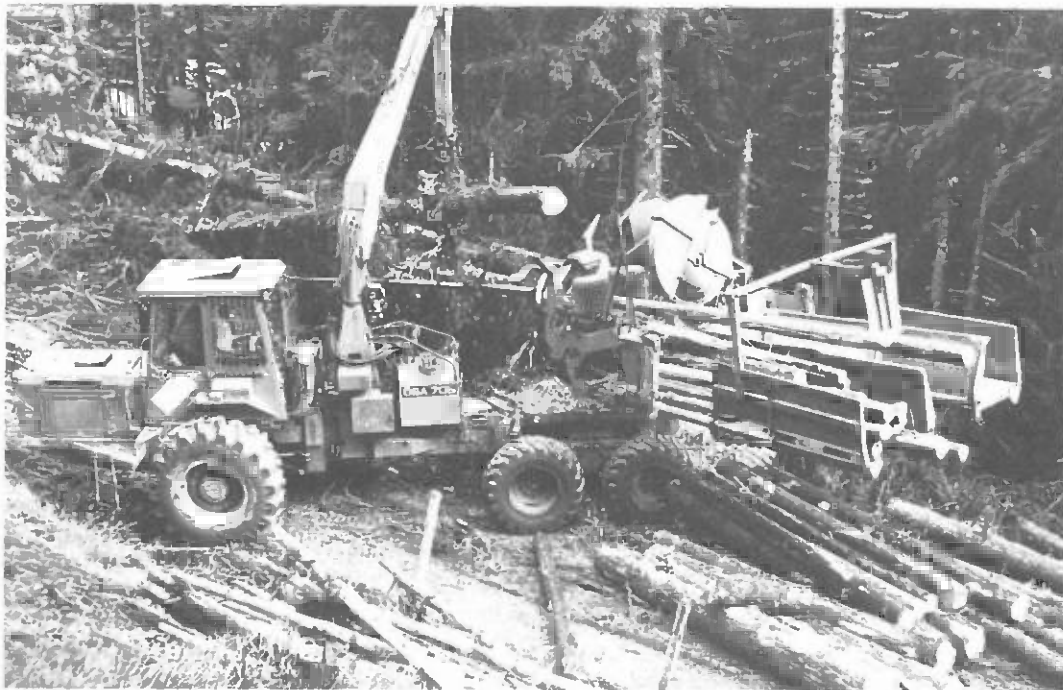
Steyr-Osa processor 705 at work delimbing and bucking (Photo: E. Pestal)
