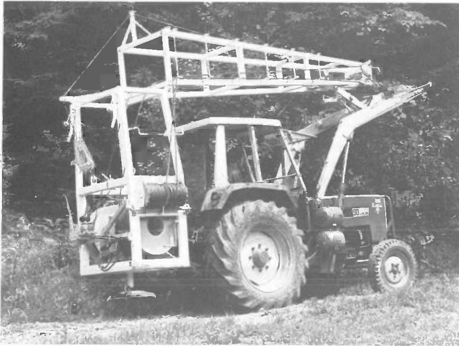
Agricultural tractor equipped with K300 cable equipment ready to be shifted to next cable-crane setting
