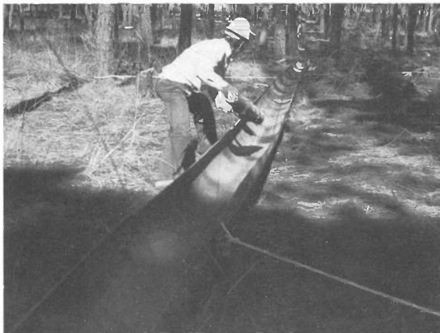
Leykam Log-Line plastic chutes of 5 m-long U-shaped sections, coupled together and used for gravity transport of timber. (Photo: R. Heinrich)
