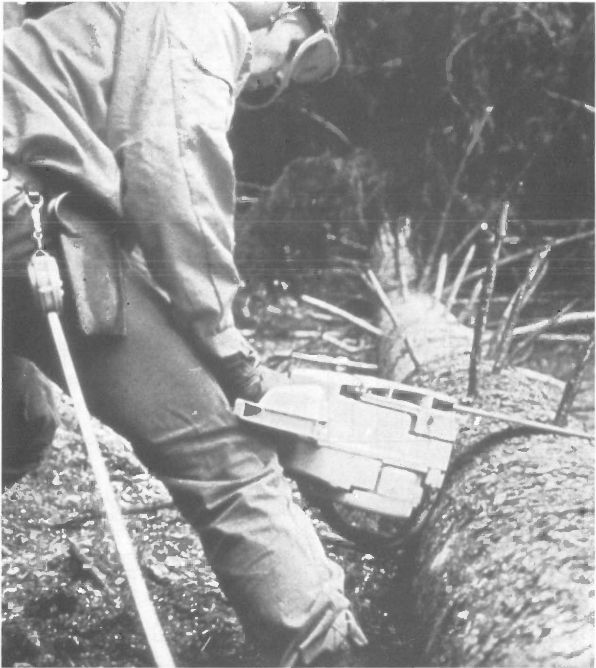
Proper delimbing is a prerequisite for efficient debarking, easy skidding and better selling opportunities (Photo: R. Heinrich)
