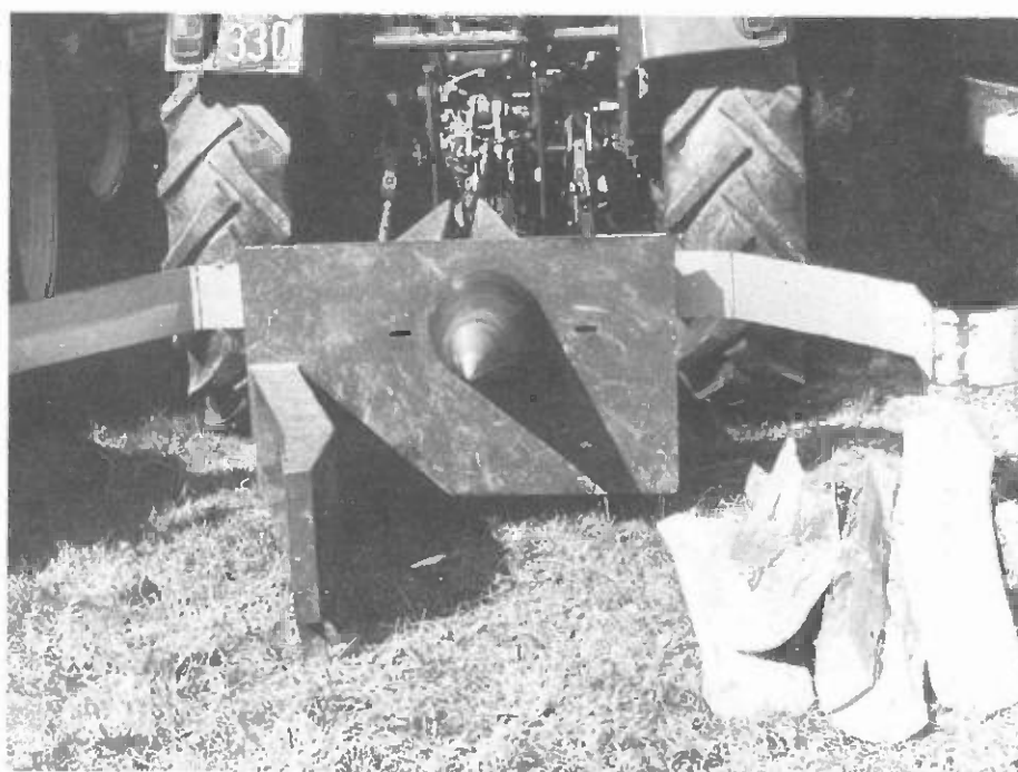
Cone-type mechanical wood splitter attached to wheeled tractor (Photo: R. Heinrich)
