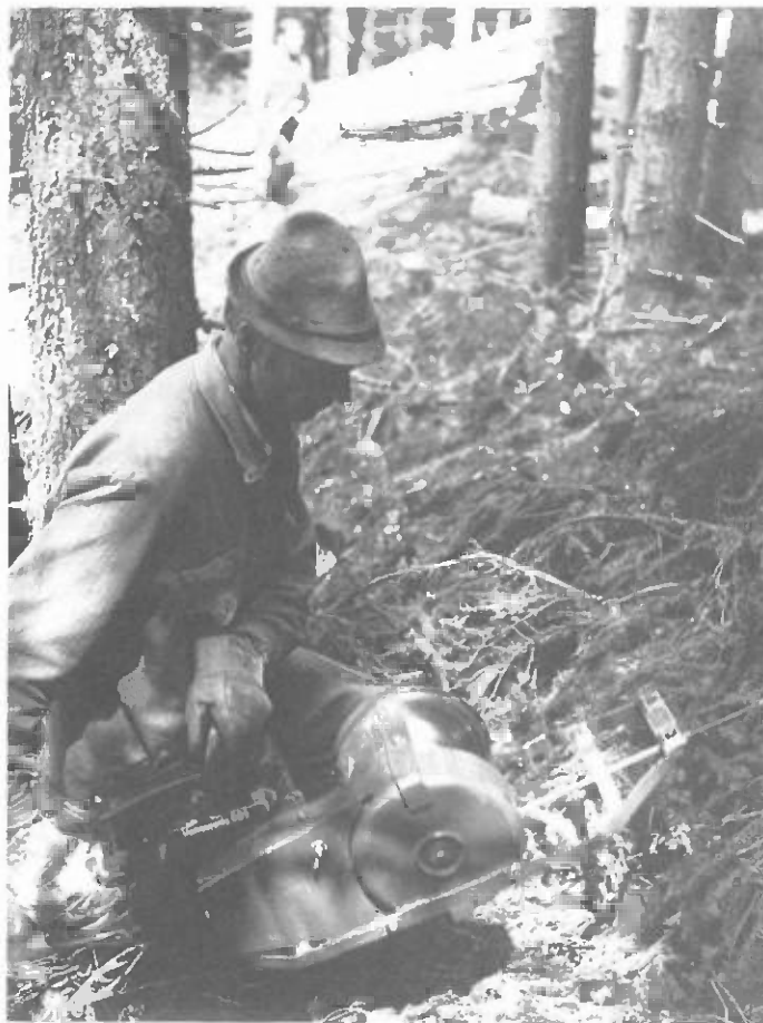
Power-saw winch for prebunching individual logs from inaccessible areas
