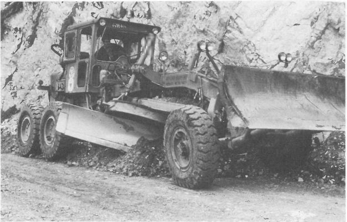
Cleaning a mountainside drain and regrading an existing forest road. (Photo R. Heinrich)
