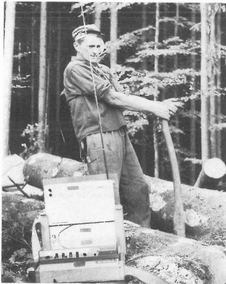
Telemetric heart-rate measurement in wood harvesting (Photo: Federal Forestry Research Institute)
