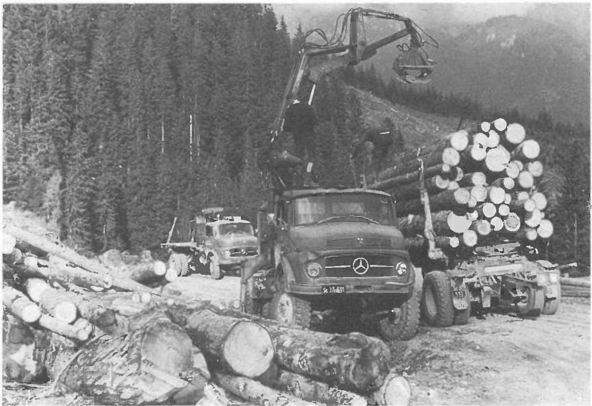
Loading of trailer and truck by truck-mounted grapple loader at the log landing. (Photo E. Pestal)
