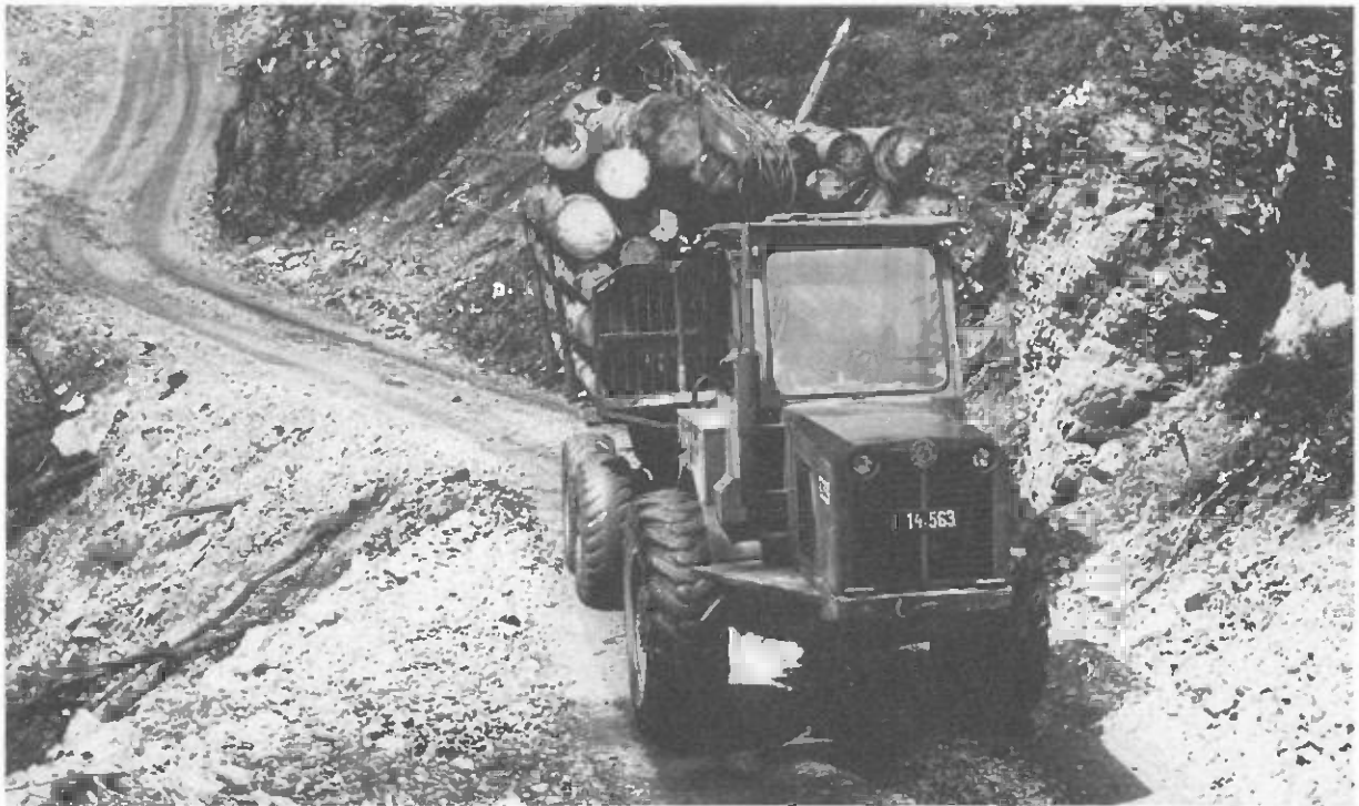
Forwarders have been used successfully in areas with wind-damaged timber and for the transport of small quantities of timber in farm forests. (Photo E. Pestal)
