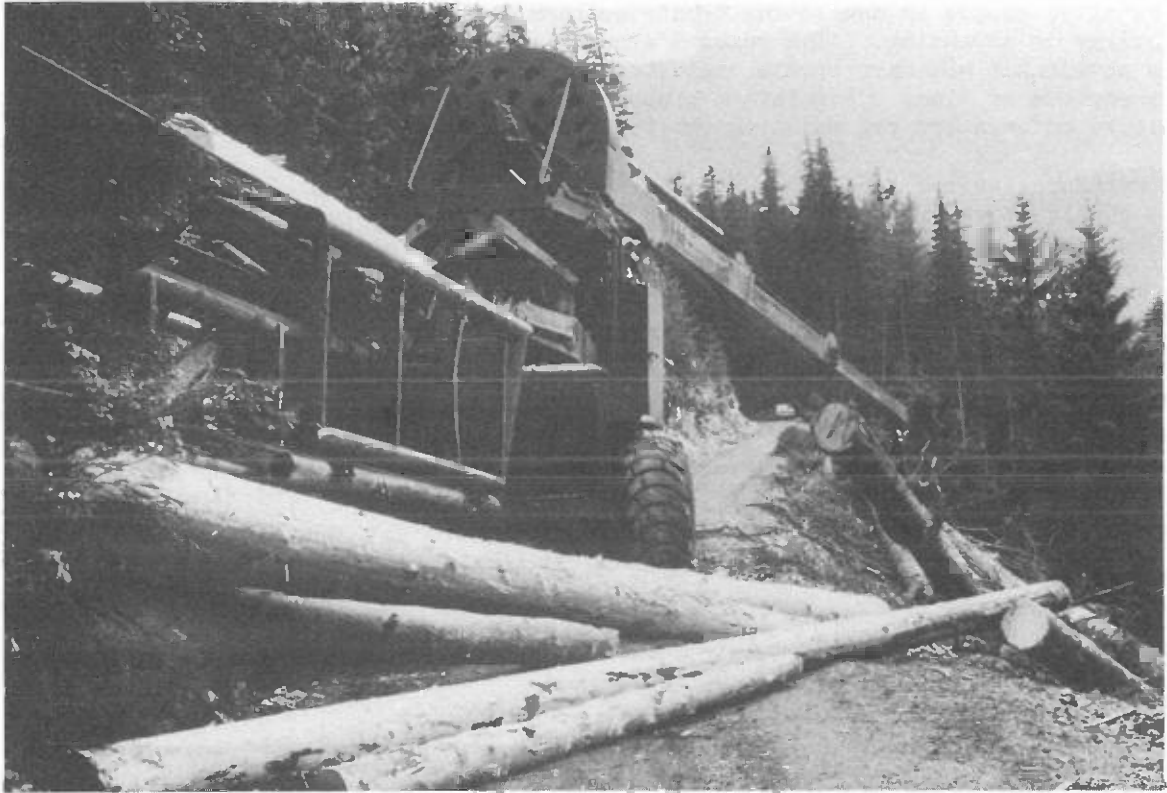
Delimber-debarker-bucker processing saw logs. (Photo R. Heinrich)
