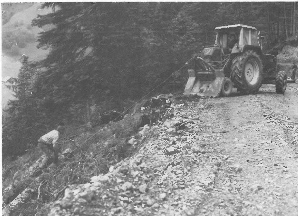
Uphill ground skidding by farm tractor with bogie. (Photo Steyr Werke)
