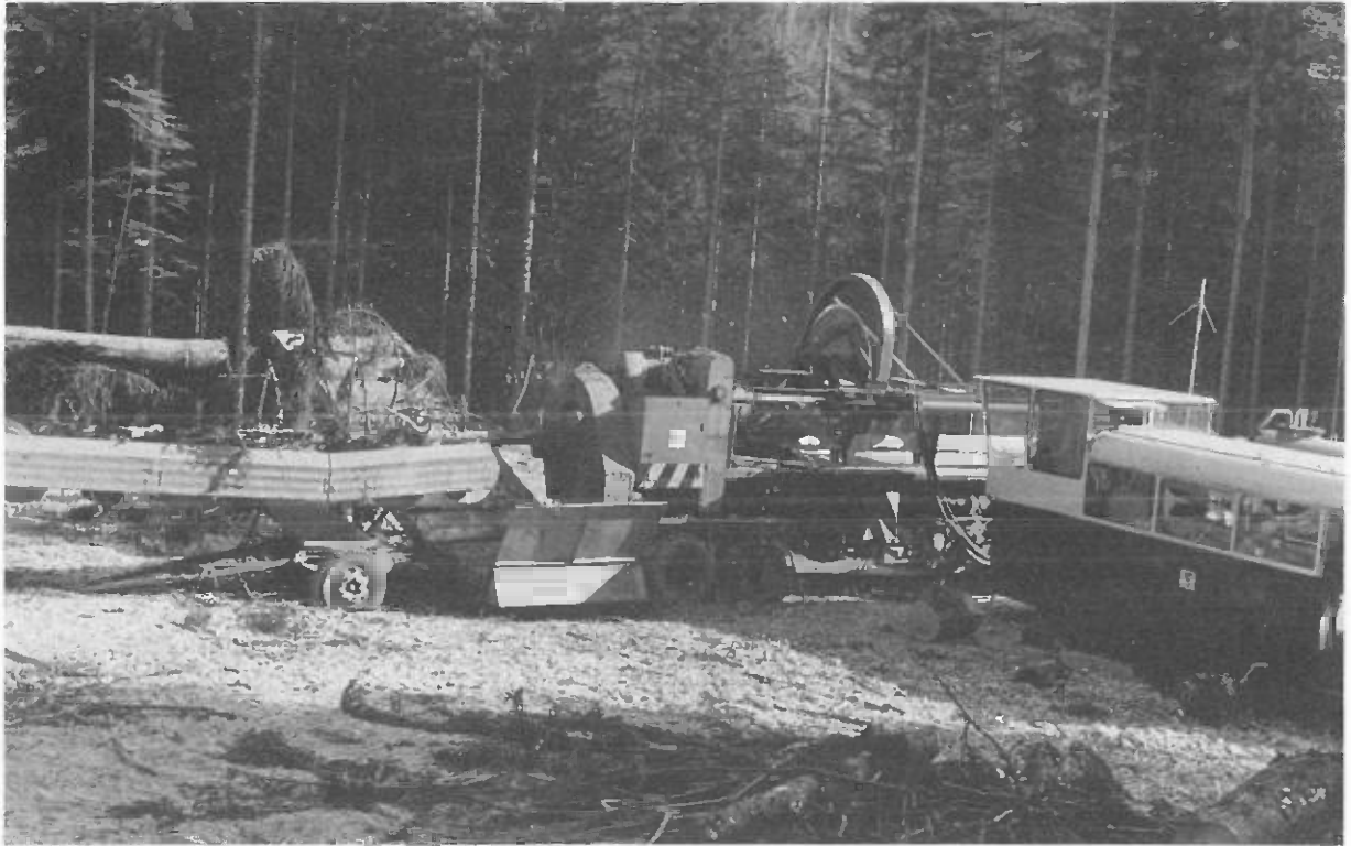
Delimber-bucker machines of the Austrian Federal Forest Enterprise have proved useful in processing wind-damaged timber (Photo E. Pestal).
