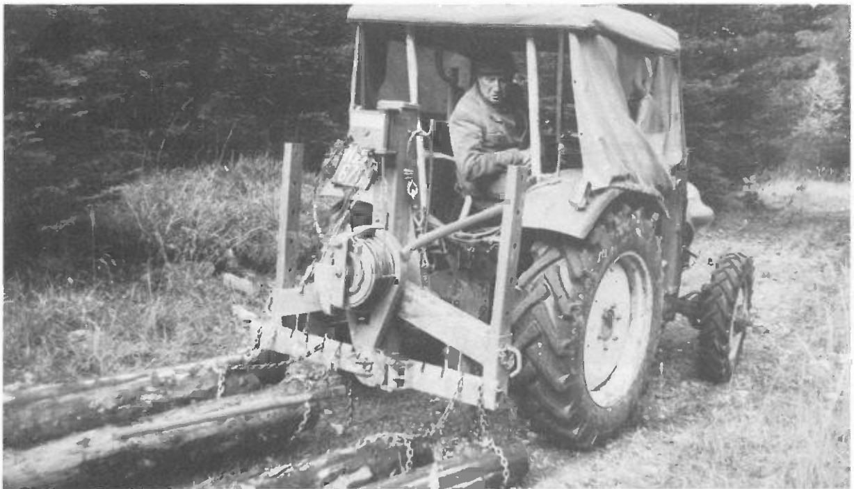
A logging winch attached to an agricultural tractor is often used for wood extraction in farm wood lots. (Photo E. Pestal)
