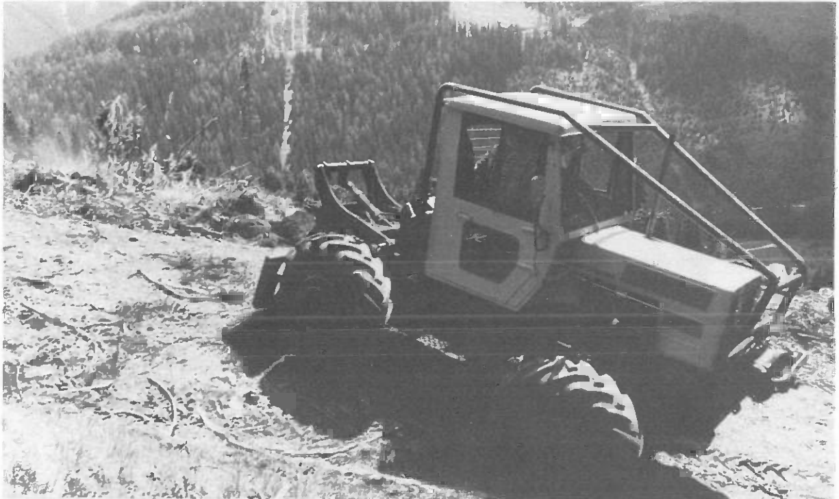
The MB-Trac fills the gap between a farm tractor and a skidder. Its cable equipment and a comfortable two-man cabin make it increasingly popular. (Photo E. Pestal)
