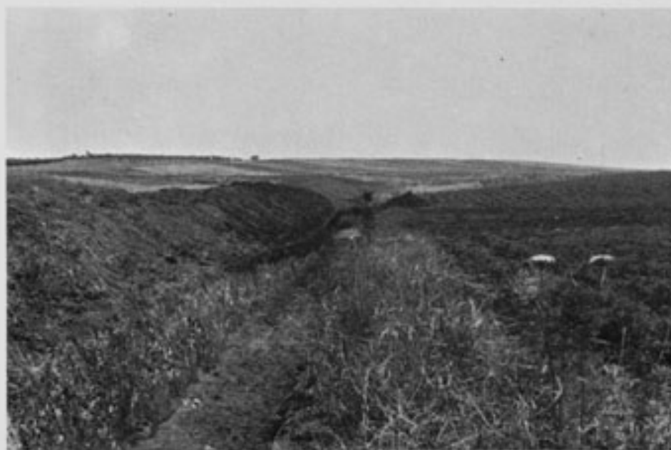
Fig. 13. Long profile cut in clayey marl, north of Montijo, Spain, showing marked change in soil characteristics. (Photo by author)
