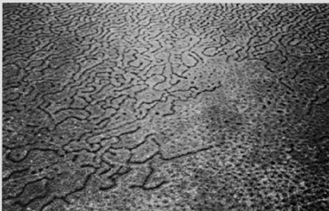
Fig. 5. This erosion type is not visible on airphotos at a scale 1:40,000. Survey is done from helicopter, annotating degree and extent of erosion on photo-mosaics. Size of erosion-gullies approx. 1m wide and deep. (Photo by author)
