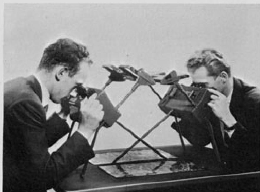
Fig. 8. Double-scanning stereoscopes for simultaneous viewing; N.V. "De Oude Delft", The Netherlands.
