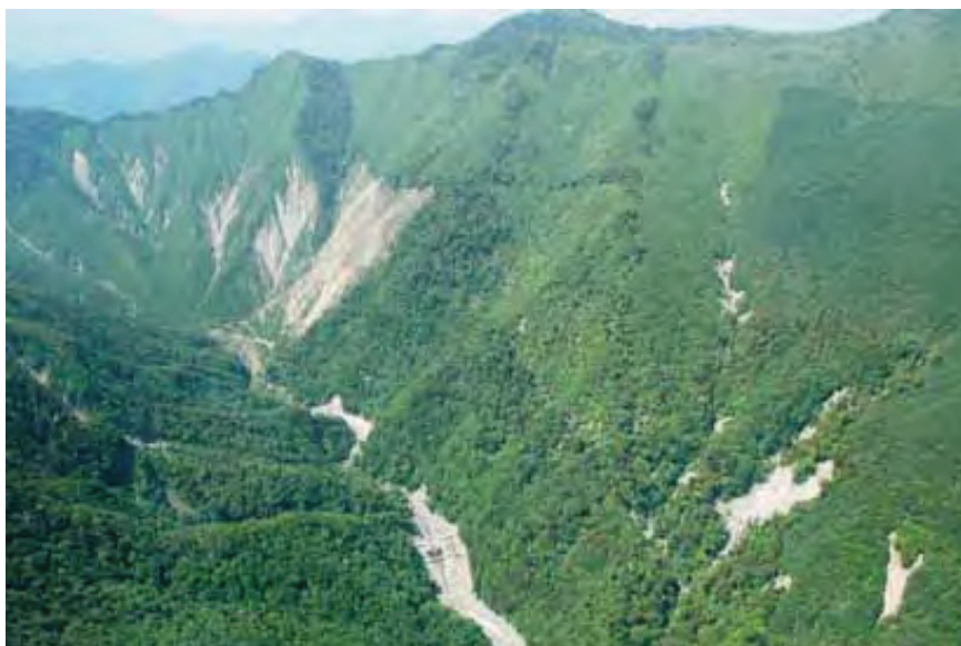
Figure 2.1. Old patterns of logging on 40-45° slopes associated with high landslide density on Kamanshi River, Yamanashi Prefecture, Southern Japanese Alps. Logging took place five years before the photo was taken. Notice clogging of the river channel and overrun check dams
