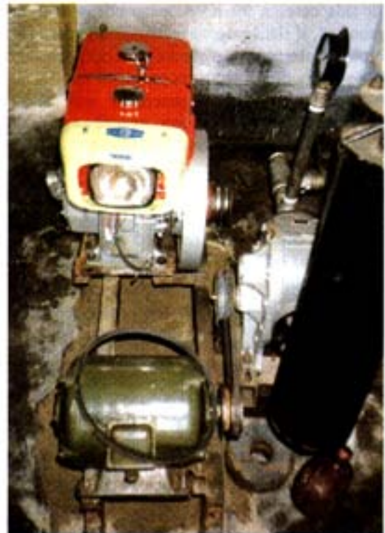
Fig. 8. Rotary lobe air blower with auxiliary diesel power.
