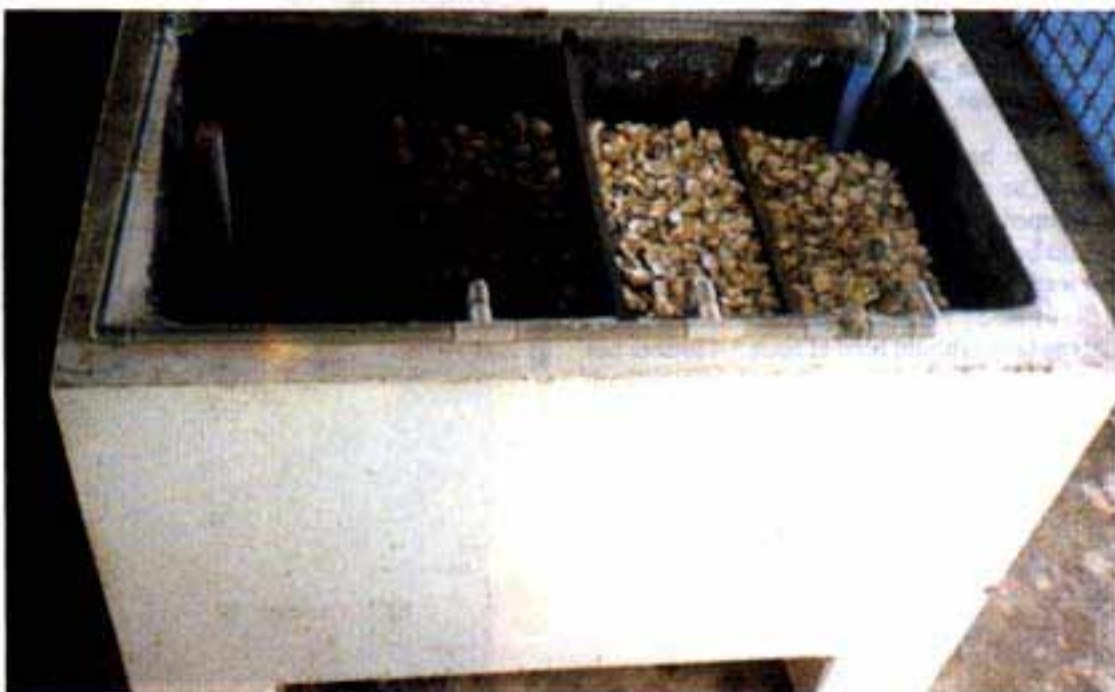
Fig. 13b Biofilter attached to larval rearing tank
