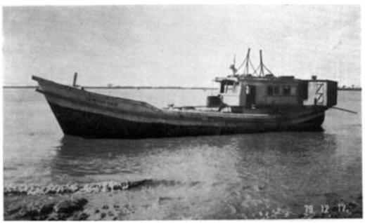
Miriam 9 (top) and Miriam 18, both fishing boats belonging to the Kalidaha fishing project, were used for the experiments to improve the large-mesh driftnets. Miriam 9 is a 12-rn wooden boat driven by a 22-H.P. engine; Miriam 18 is a 13 m ferro-cement boat with a 33 H.P. engine.
