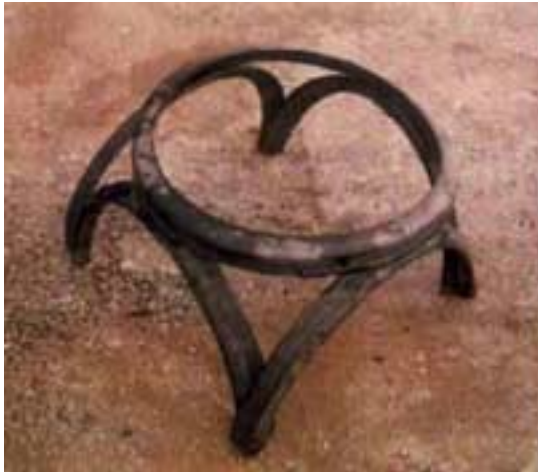
The stand of a local-type garbage bin made from truck tyres
