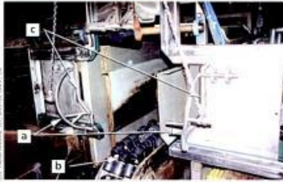
PHOTO 7.2 Upright cattle restraint with monorail conveyor a) Chin lift, b) Monorail, c) Neck restraint
