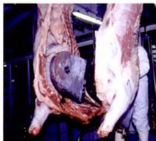
PHOTO 8.46 Splitting the carcass in the medial plane by power
