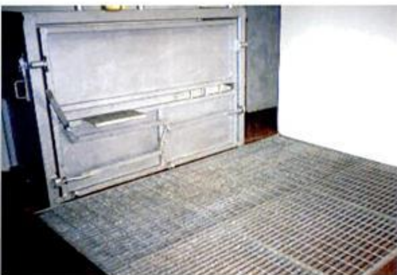
PHOTO 10.2 GOOD PRACTICE: cattle stunning pen with raised grid to keep stunned animals off the floor and reduce coat contamination
