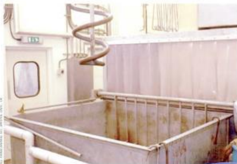
PHOTO 10.5 A scald tank and associated dehairer for pigs
