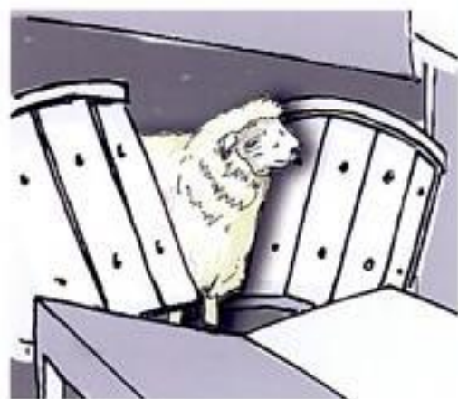
FIGURE 7.1 V-type restraint conveyor for sheep
