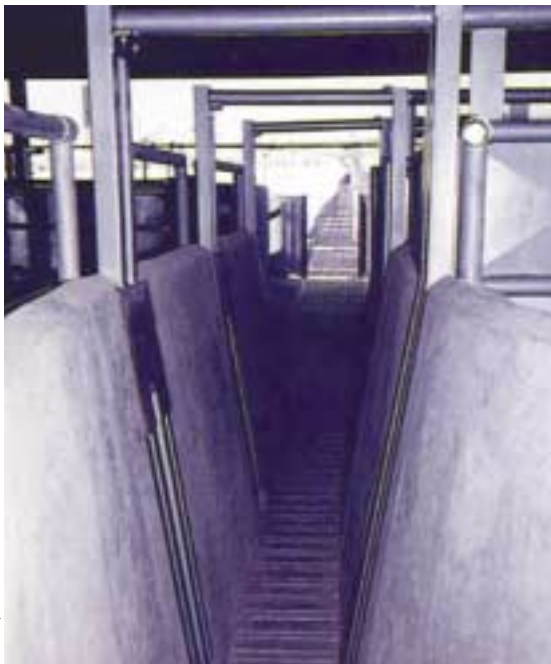
PHOTO 5.5 GOOD PRACTICE: clearly lit raceway for cattle from pen to stunning area
