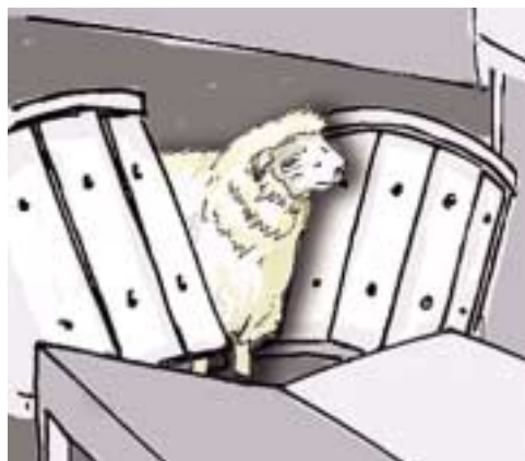
FIGURE 7.1 V-type restraint conveyor for sheep
