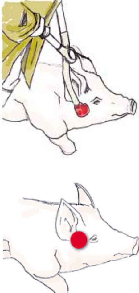
FIGURE 7.3 GOOD PRACTICE: optimum tong position for head-only electrical stunning of pigs
