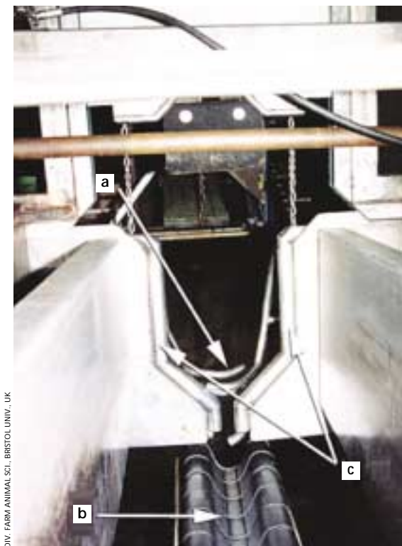
PHOTO 7.3 Upright cattle restraint with monorail (internal view) a) Chin lift, b) Monorail, c) Neck restraint
