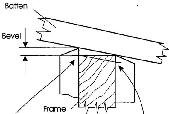
Mark gap between batten and frame = bevel on a stick and transfer to the other side of the frame.
