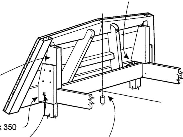
2 The centerline on the transom must be aligned with the centerline string
