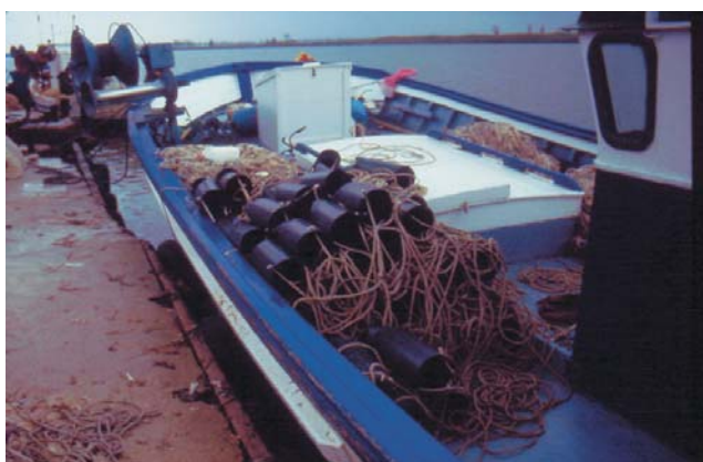
54) PVC pipe pots linked by a line for Octopus vulgaris fishery - Deltebre, Catalonia (M. Demestre)
