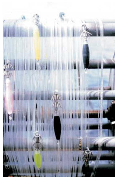
60) Soft body (green) and hard body (black) squid jigging hooks on reel - Japan (C.F.E. Roper)
