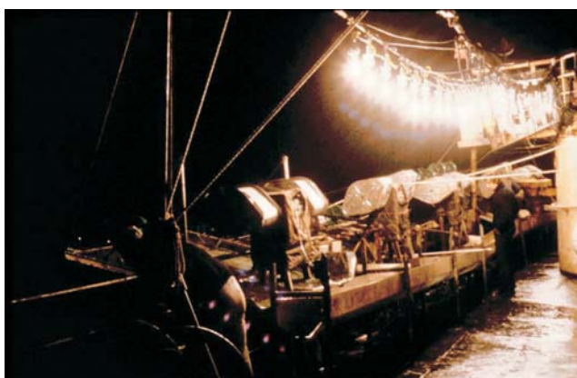
50) Squid jigging machines at night - Japan (W.F. Rathjen)
