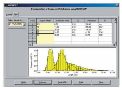
Fig. 4.12. NORMSEP user interface in decomposing composite distributions.
